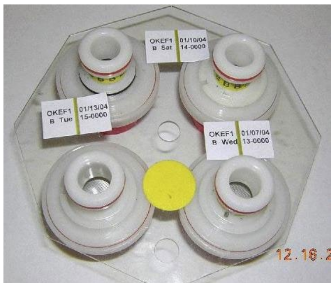
Figure 4. Sample cartridge for the 2B module (yellow sticker) with four cassettes. Only three of the cassettes contain sample filters (indicated by the three labels).
