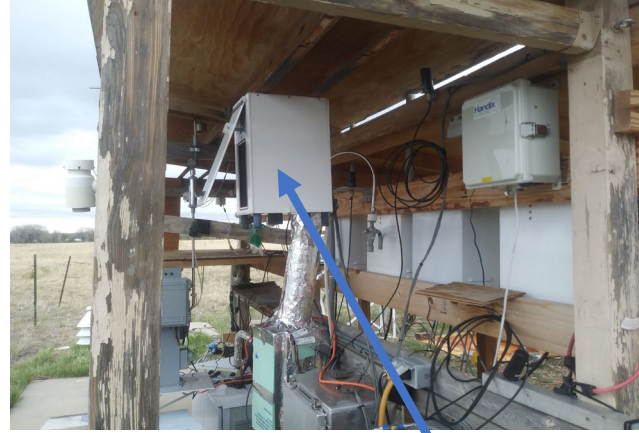
Side View – Open air Nephelometer
