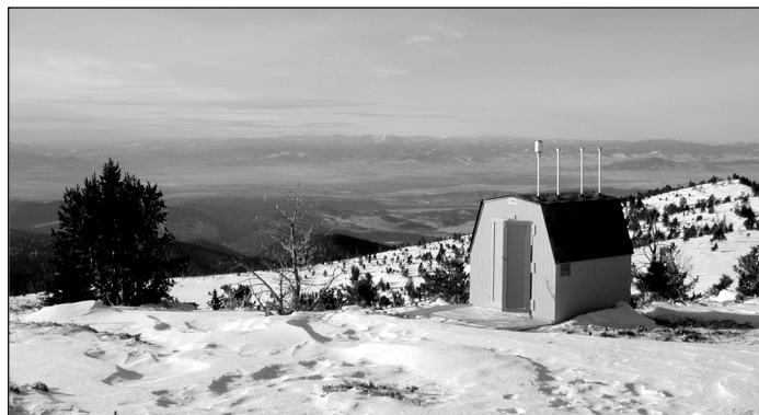
Gates of the Mountains monitoring station in the Helena National Forest is located atop Hogback Mountain. The station is equipped with an IMPROVE aerosol sampler and a remote digital camera system.
