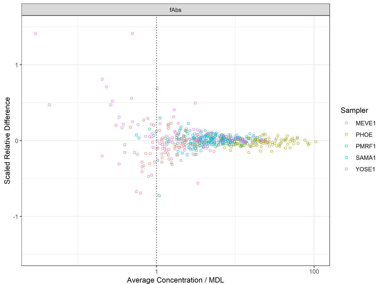
Figure 19: Scaled relative difference for optical absorption measurements at sites with colocated modules across the IMPROVE network (2017). Dotted vertical line indicates method detection limit.
