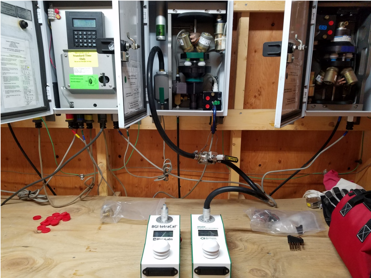
Figure 6 Photo showing sampler flow rate and vacuum checks during audit.
