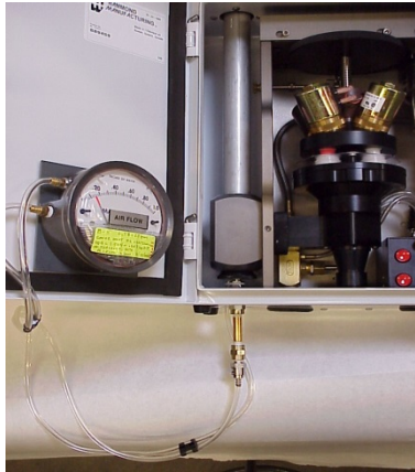
Figure 2. Inserting the Probe into the Tee
