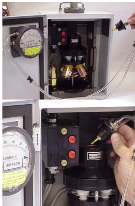
Figure 6. Placing the Probe in Module "D"
