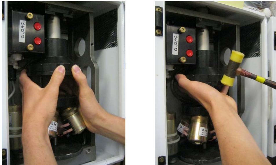
Figure 7. Removing the Bottom Lid of Module "D"
