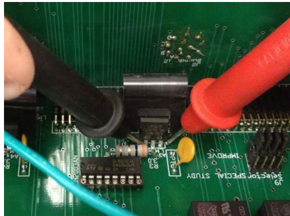
Figure 4. Checking Voltage Regulator
