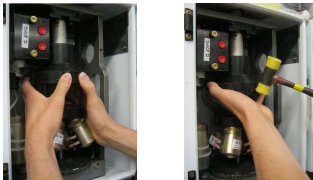
Figure 7. Removing the Bottom Lid of Module "D"
