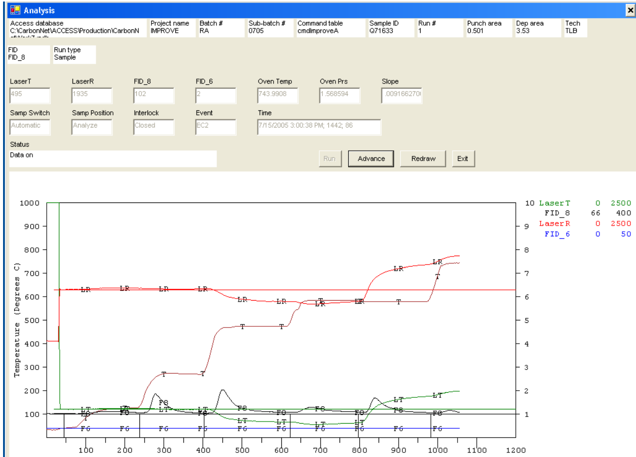
Figure 4-2b. The Analysis Screen during Sample Analysis for DRI Model 2001 Thermal/Optical Carbon Analysis Program.
