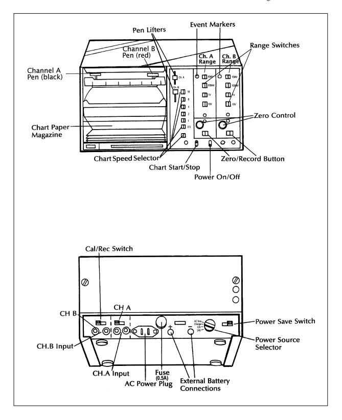
Figure 4-1. Strip Chart Component Diagram.
