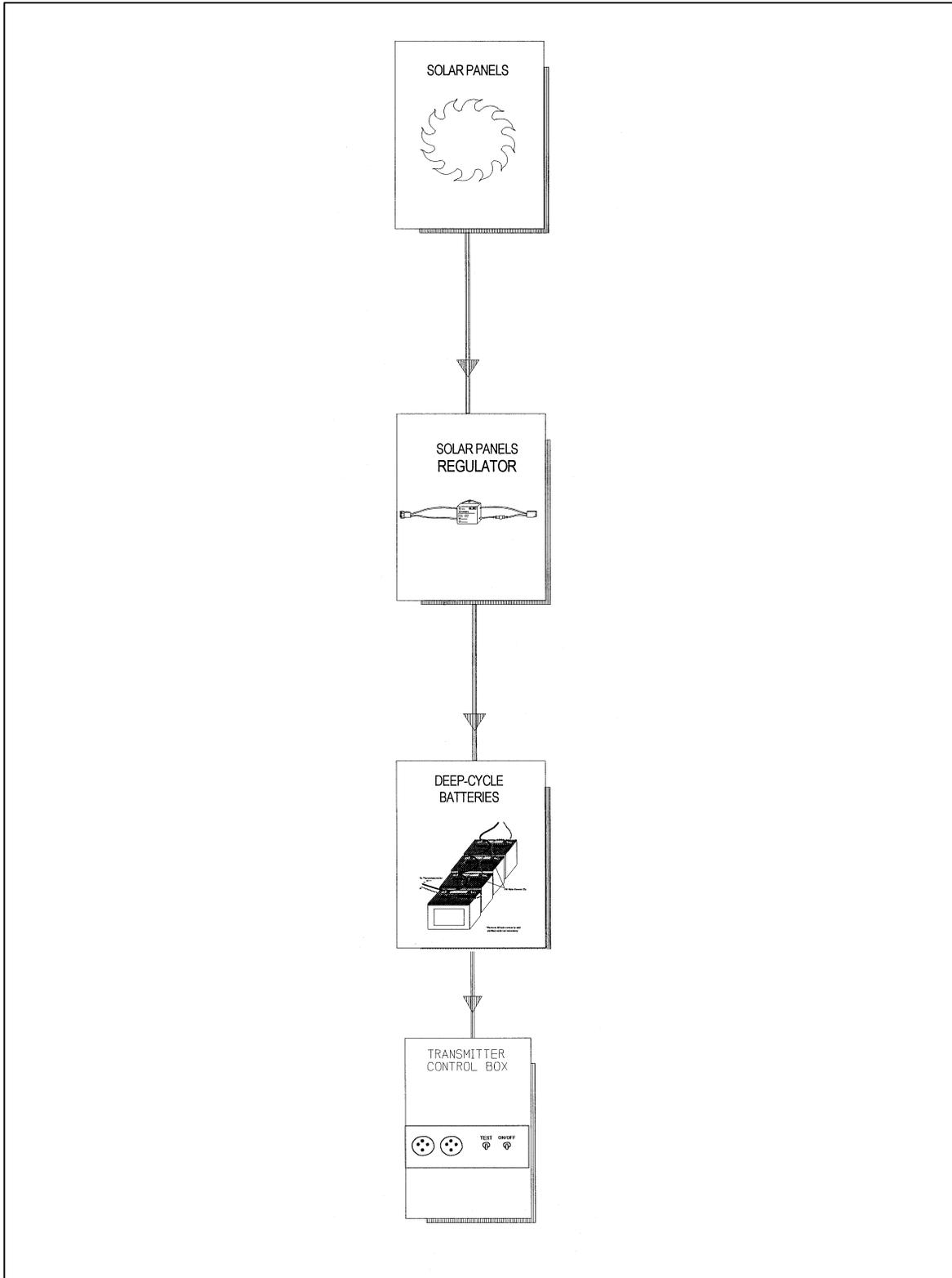
Figure 4-26. Transmitter Station Solar Power (DC) Configuration Diagram.
