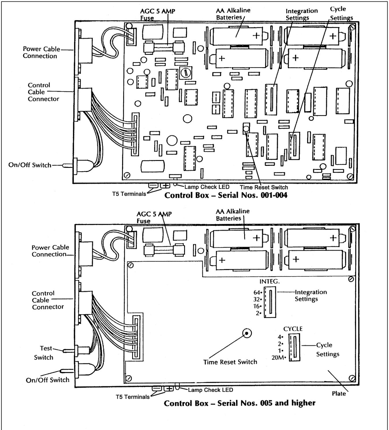
Figure 4-3. Transmitter Control Box Diagram.
