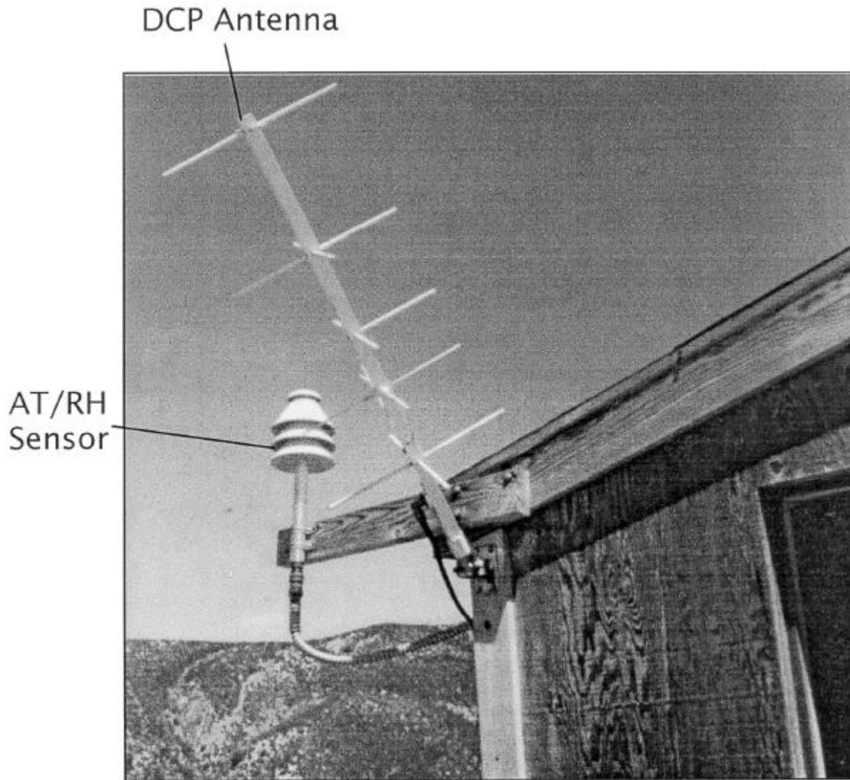
Figure 4-17. Mounted AT/RH Sensor and DCP Antenna.
