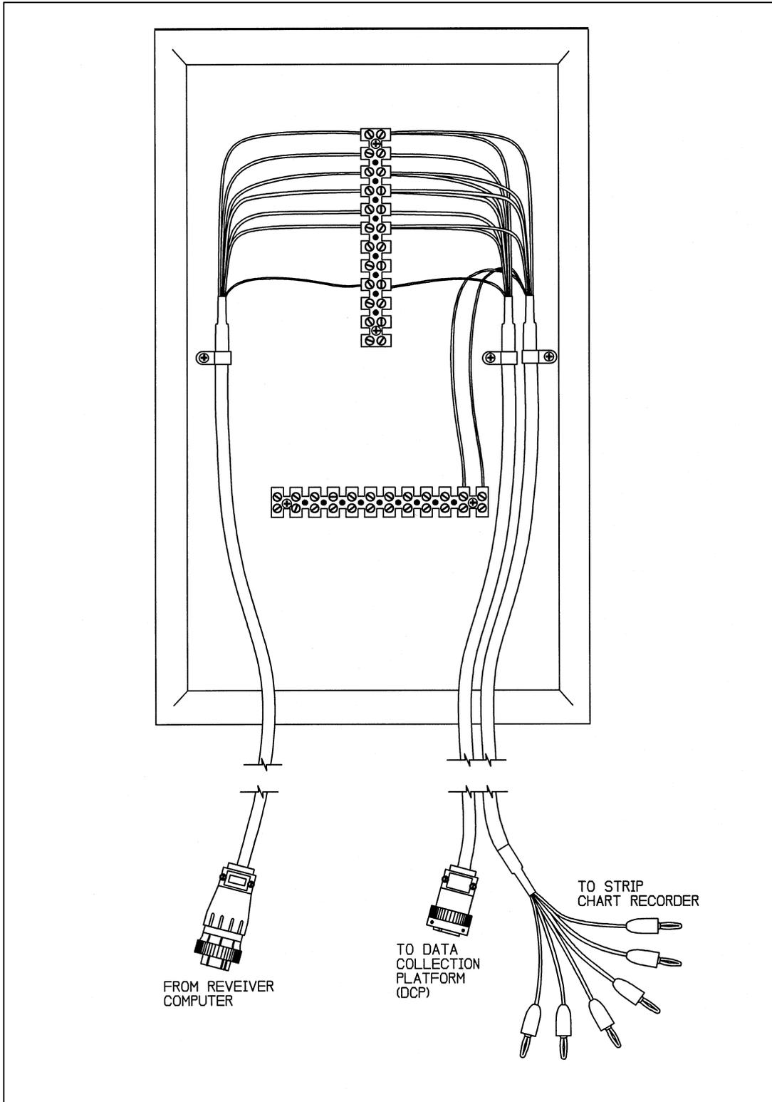
Figure 4-8. Terminal Strip Board With Cable Connectors Diagram.
