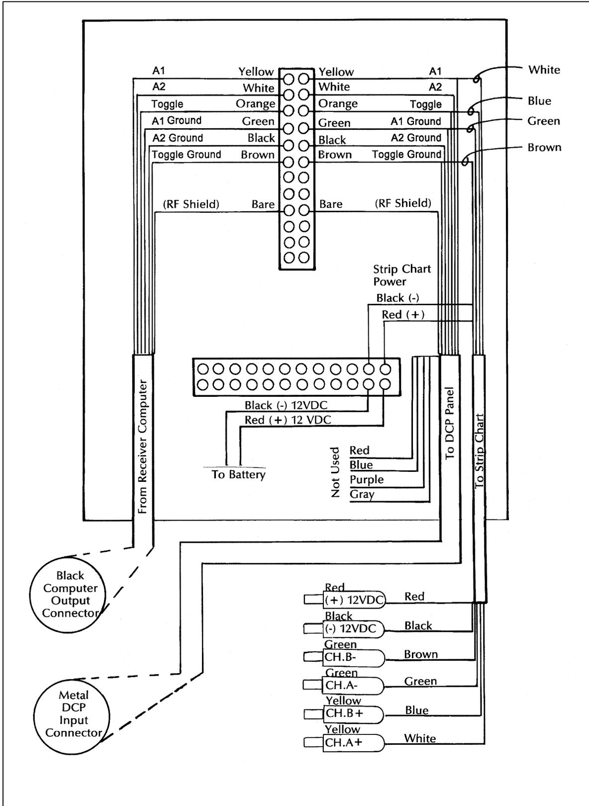
Figure 4-9. Terminal Strip Wiring Diagram.
