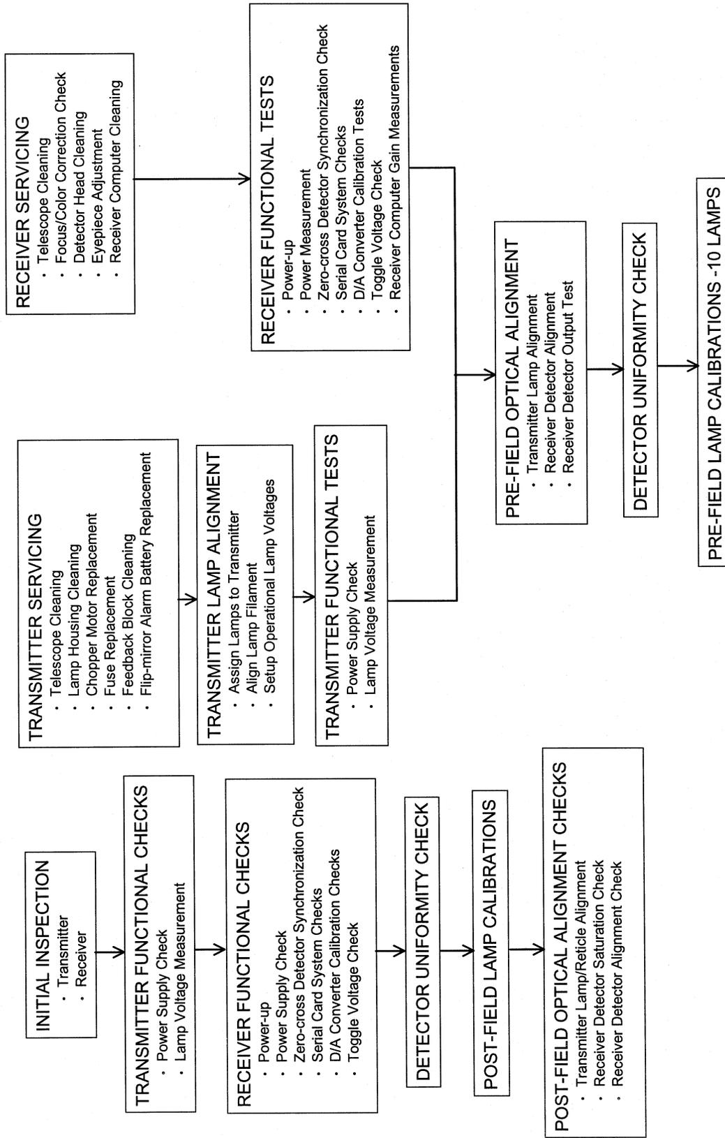
Figure 4-1. Flowchart of Transmissometer Annual Maintenance Procedures.
