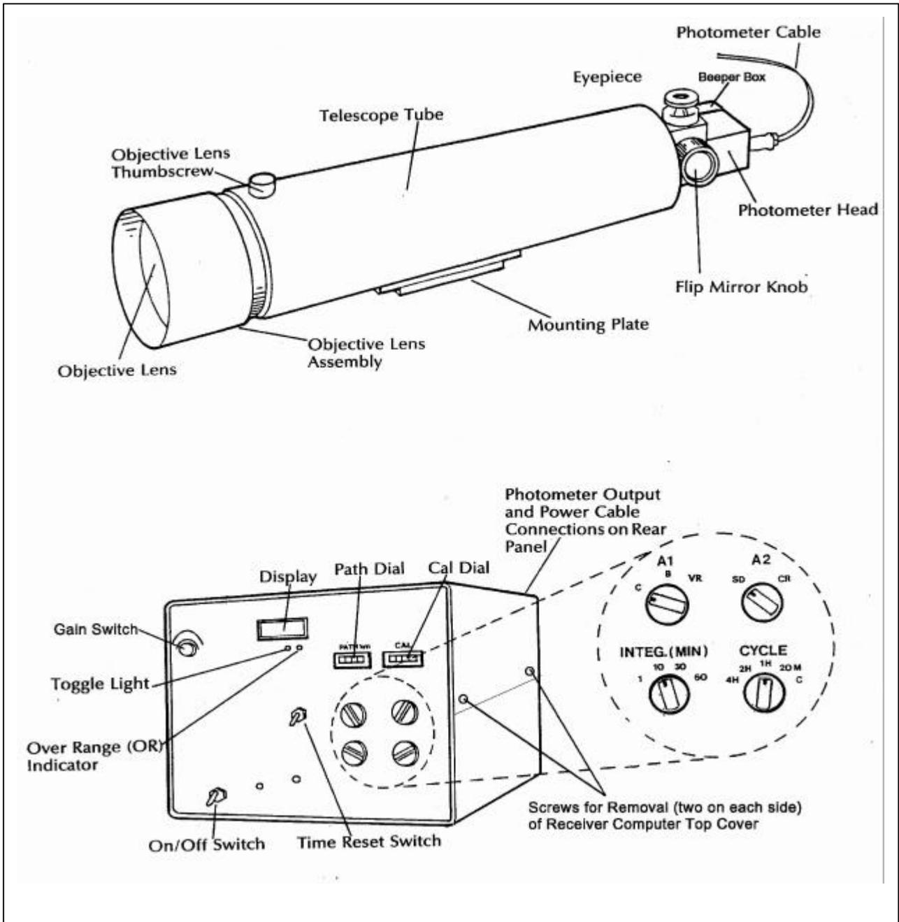
Figure 4-5. Receiver Component Diagram.
