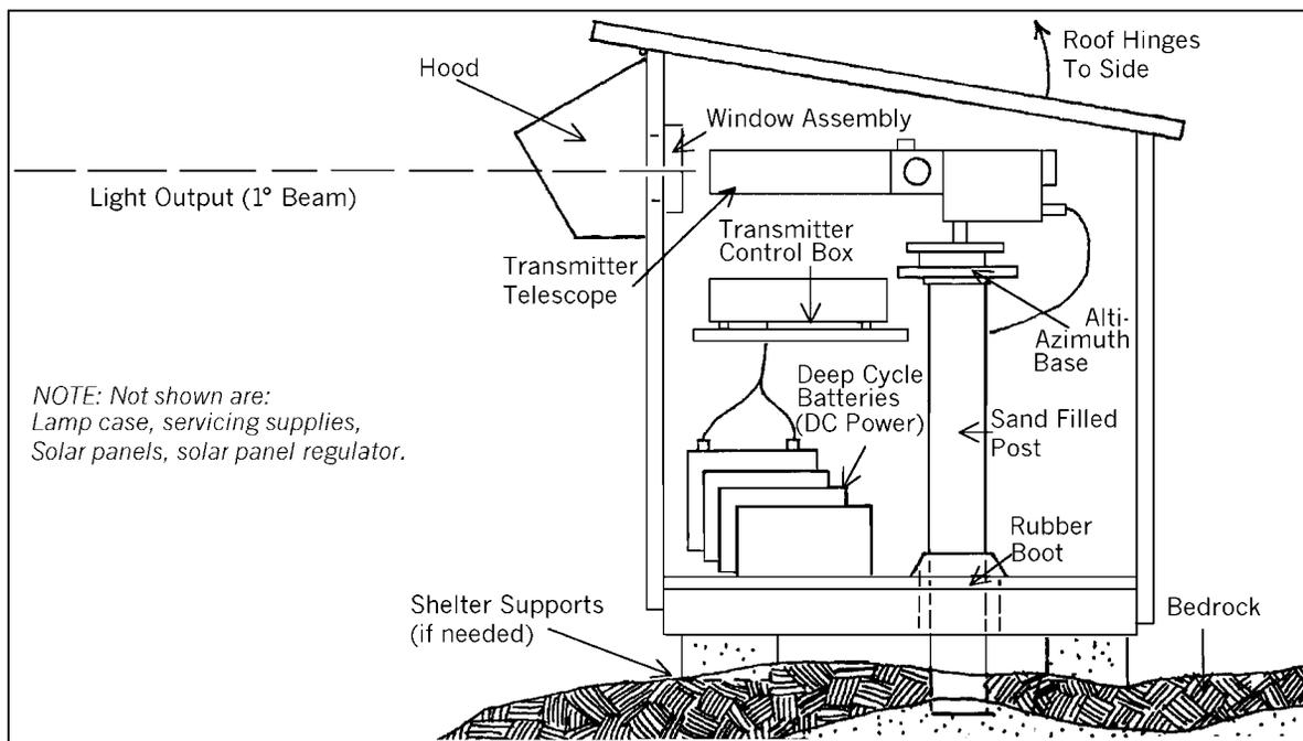
Figure 4-1. Typical Transmissometer Configuration - IMPROVE Network.
