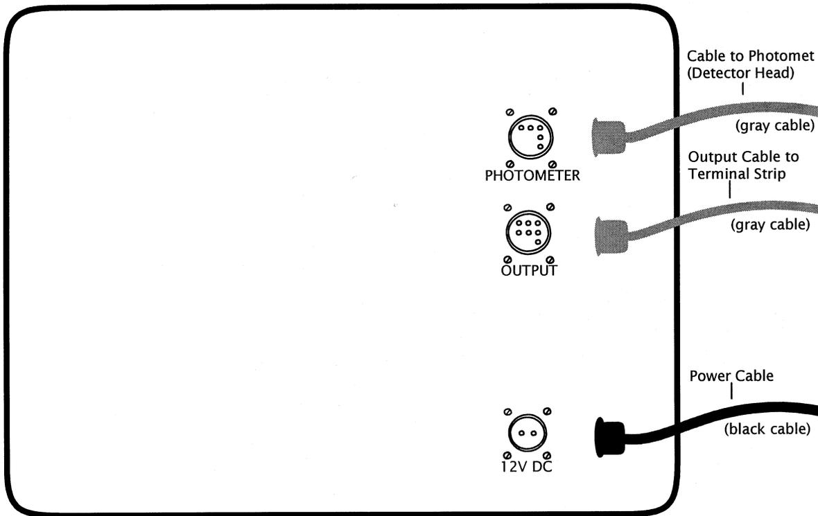
Figure 4-6. Receiver Computer Cable Connections Diagram.
