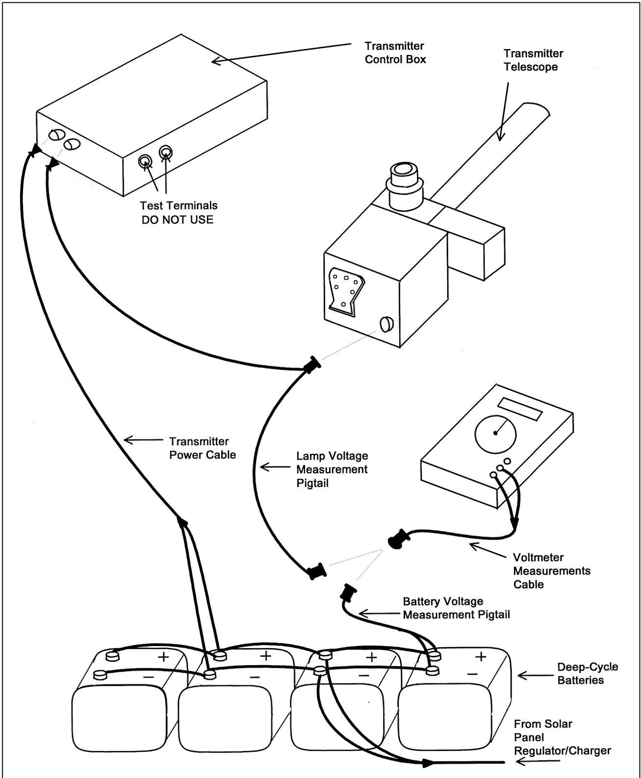
Figure 4-3. Transmitter Components Connection Diagram.
