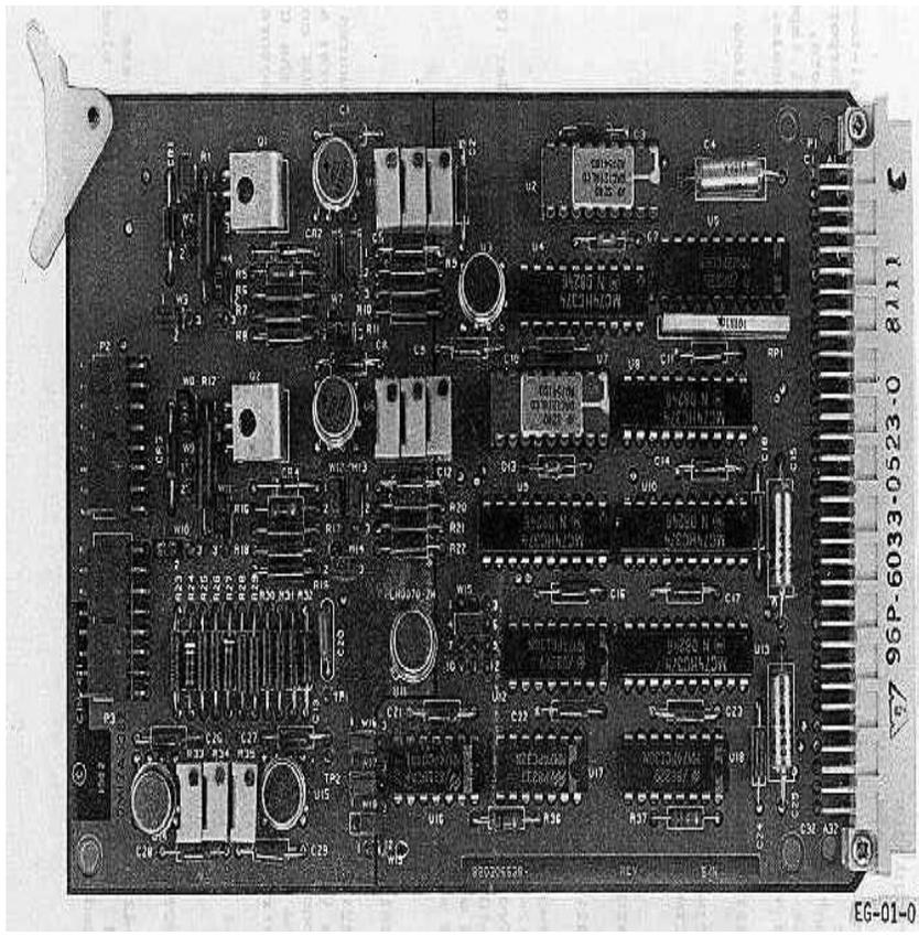
Figure 4-13. CIMBUS D/A Converter Circuit Board Components Diagram.
