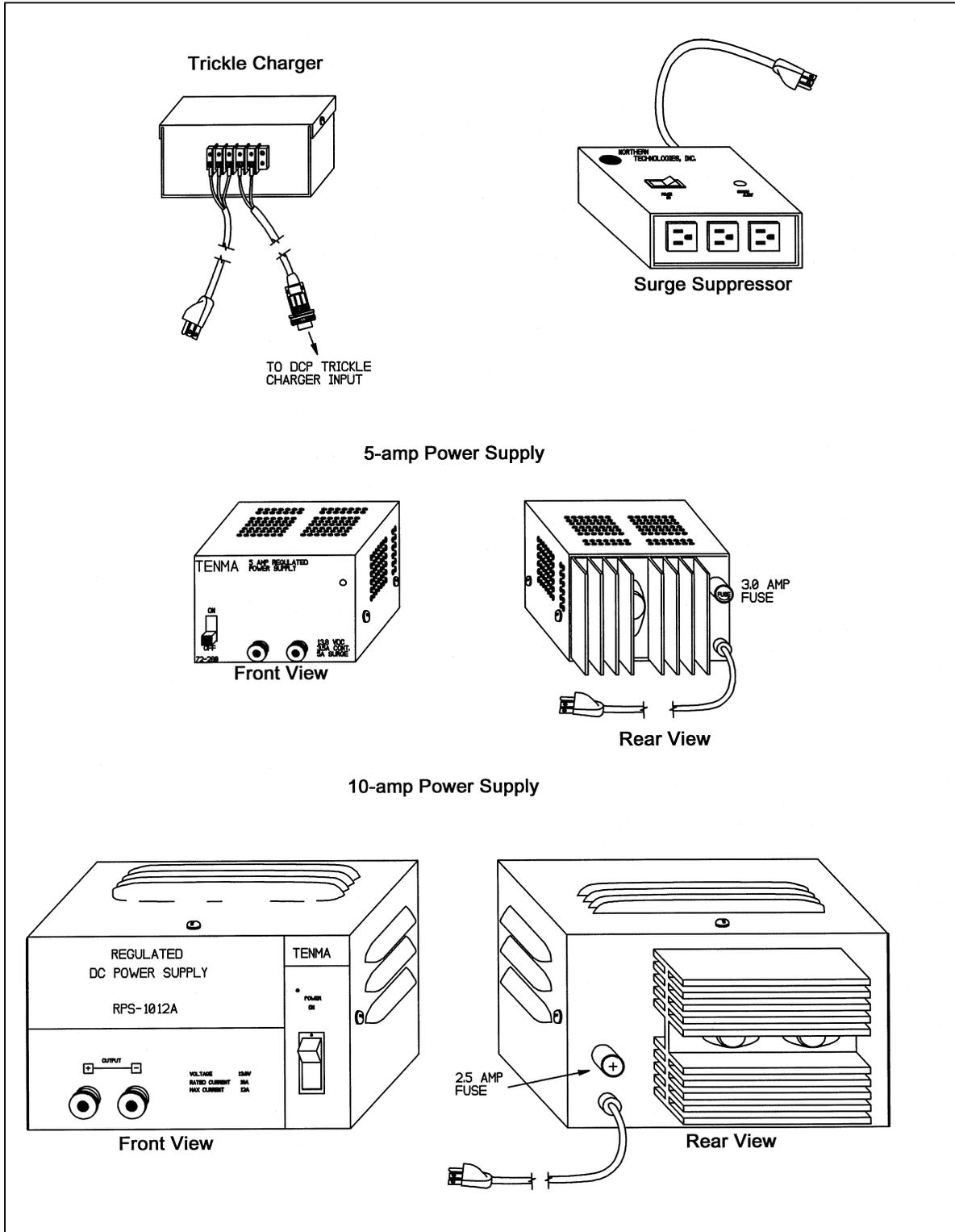
Figure 4-21. Line Power (AC) Components Diagram.
