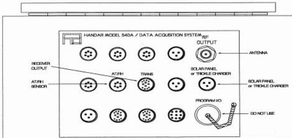
570 DCP CABLE CONNECTION & DISPLAY DIAGRAM
