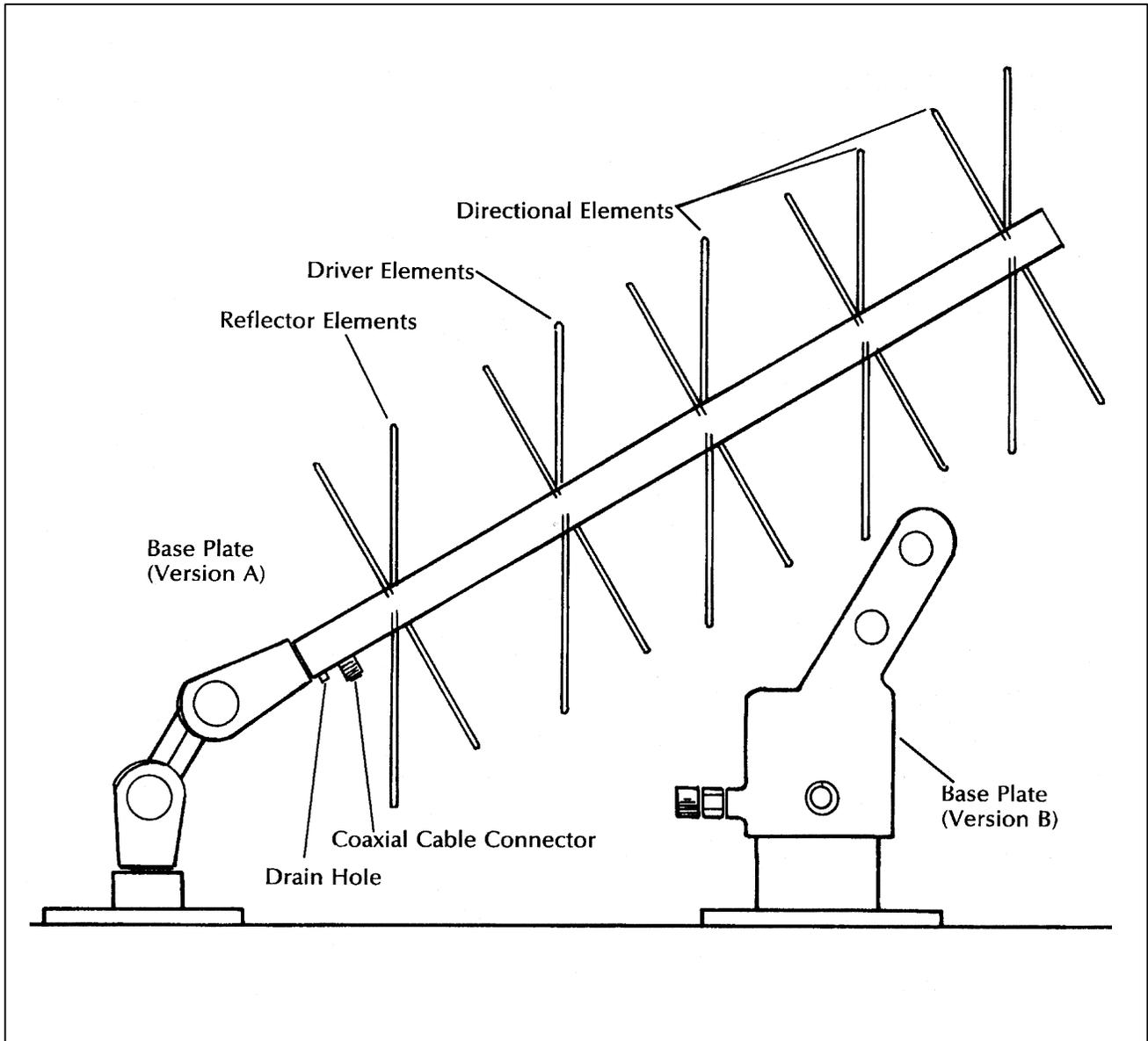
Figure 4-13. DCP Antenna Component Diagram.
