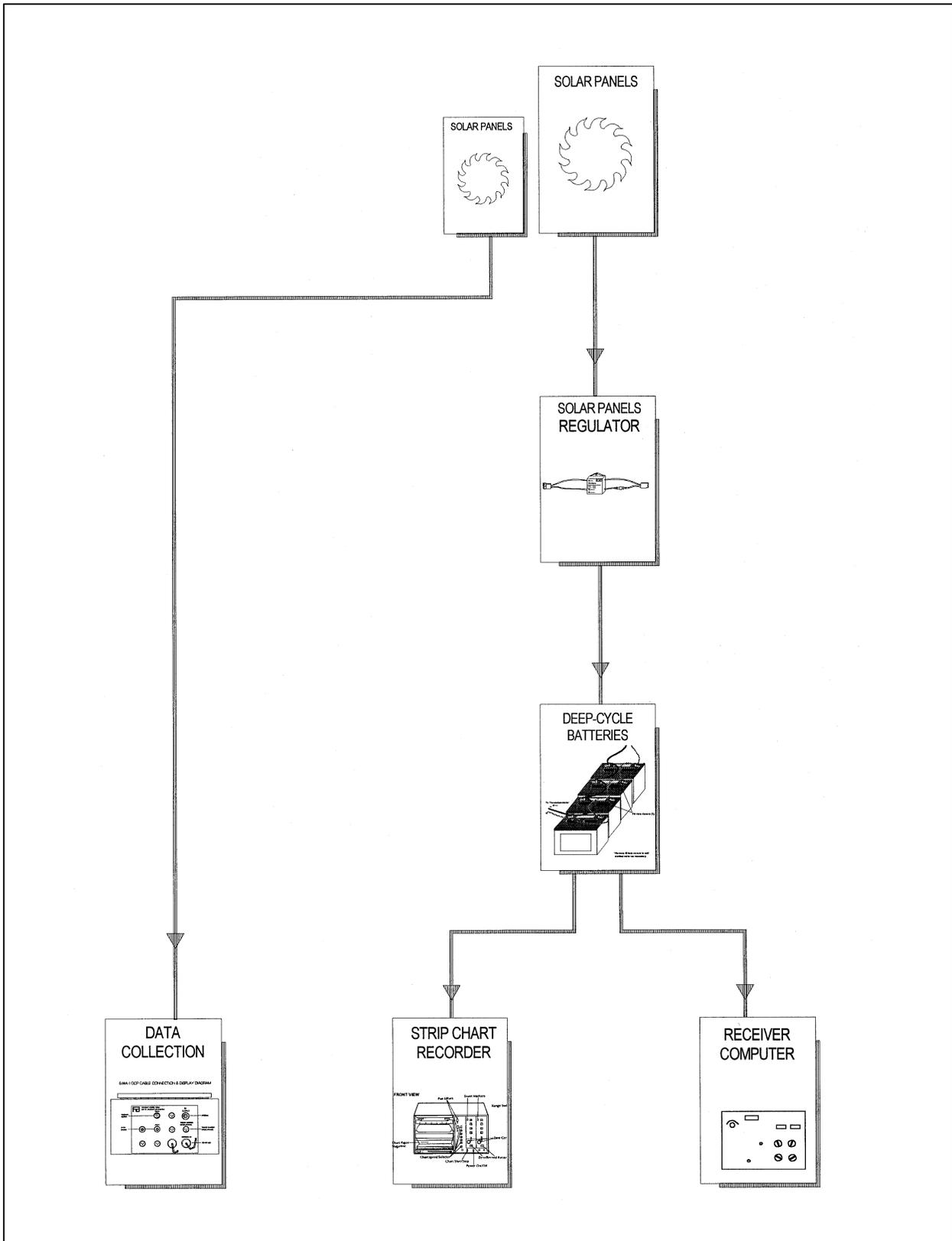
Figure 4-25. Receiver Station Solar Power (DC) Configuration Diagram.
