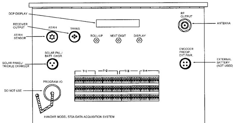
Figure 4-5. DCP Cable Connection and Display Diagram.
