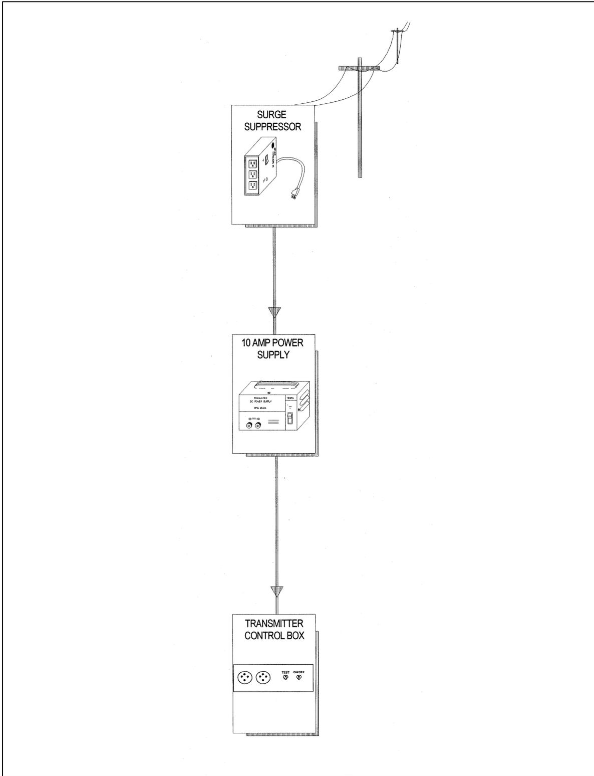
Figure 4-23. Transmitter Station Line Power (AC) Configuration Diagram.
