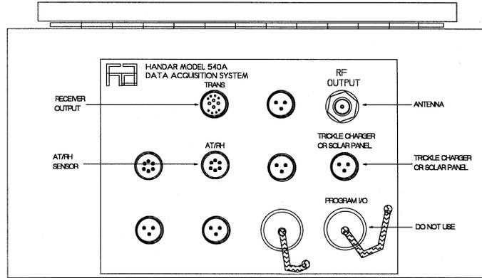
540A-2 DCP CABLE CONNECTION & DISPLAY DIAGRAM
