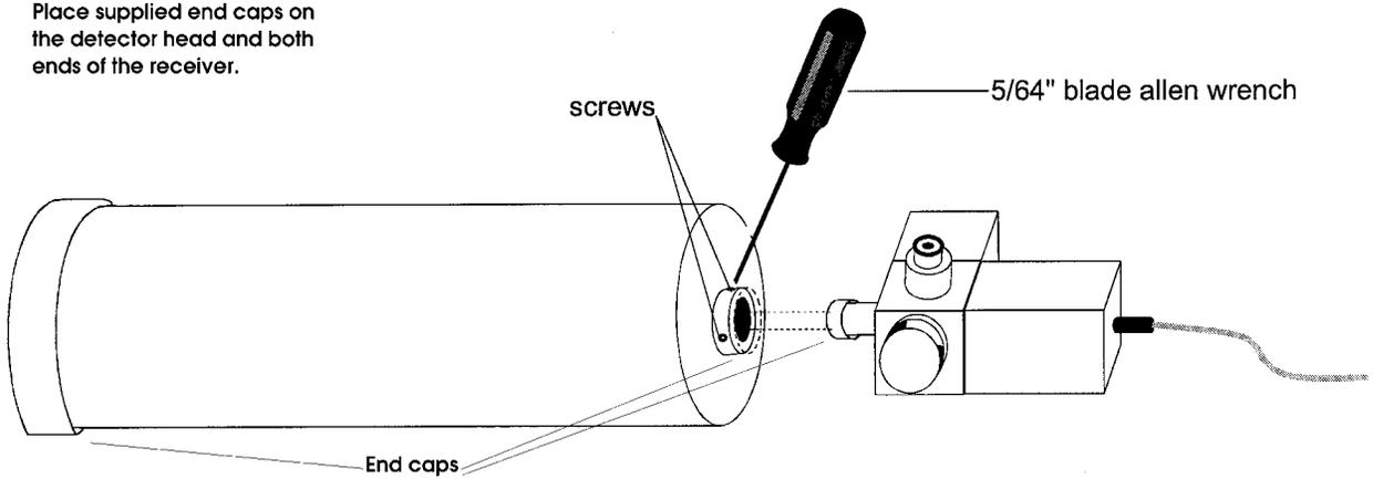
Figure 4-2. Removal of Receiver Detector Head.
