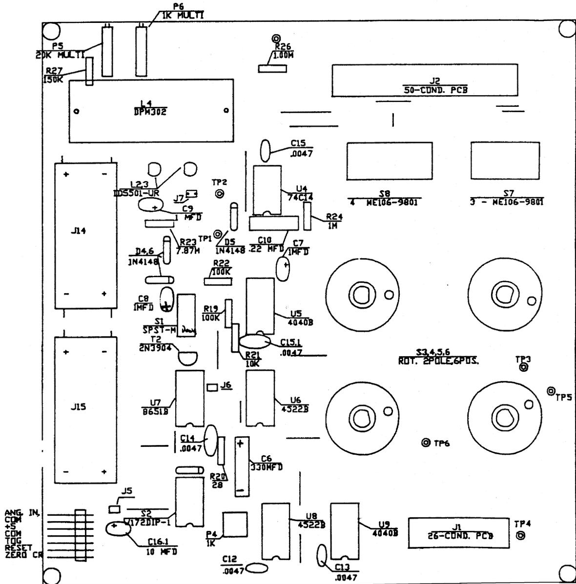
Figure 4-4. Receiver Computer Front Panel Circuit Board Components Diagram.
