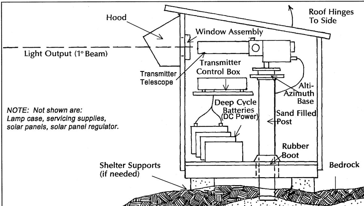
Figure 4-19. Monitoring Component Diagram (Receiver and Transmitter Shelters).
