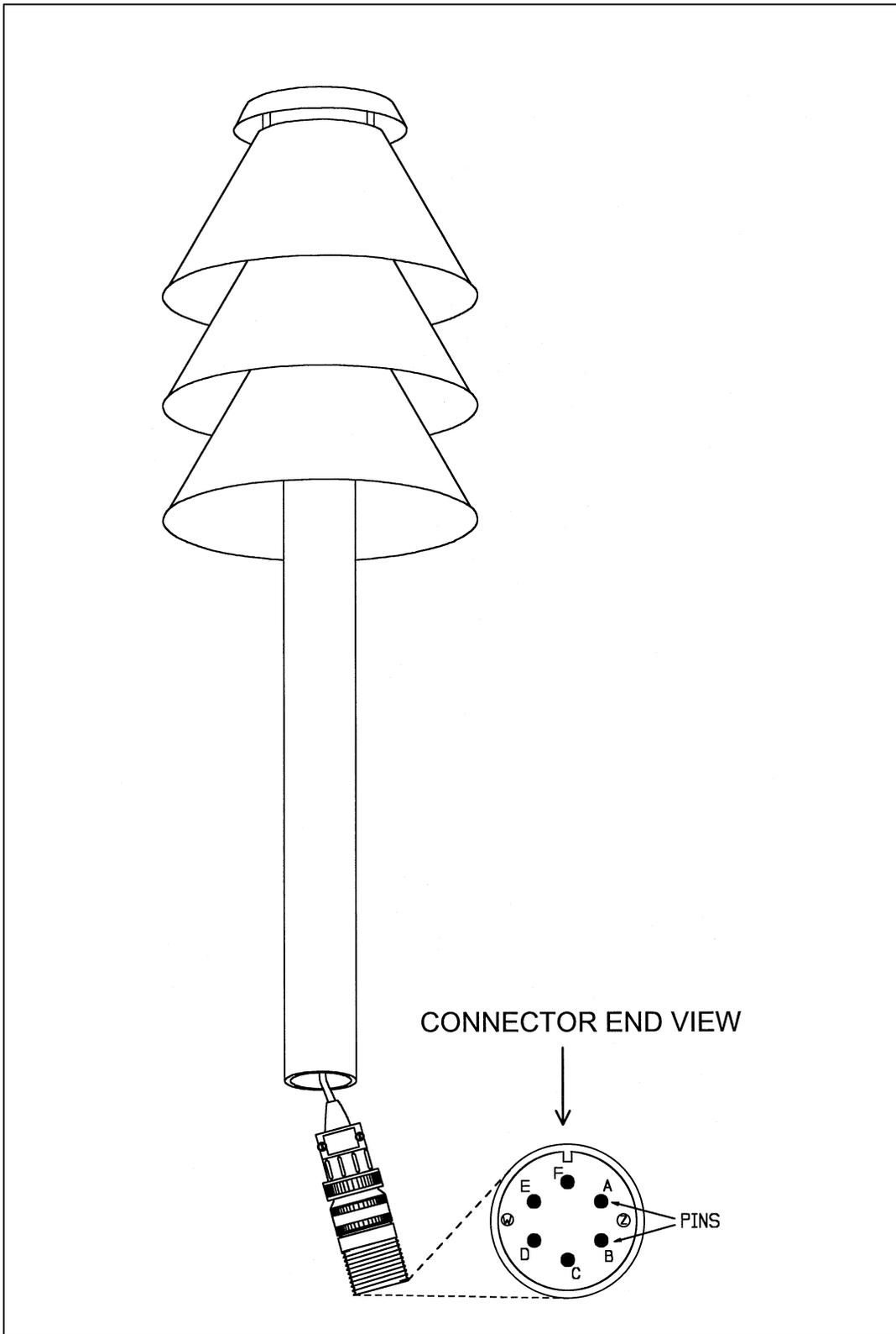
Figure 4-16. AT/RH Sensor and Cable Diagram.
