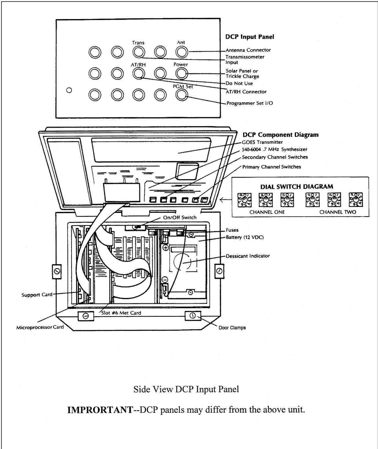
Figure 4-11. DCP Component Diagram.
