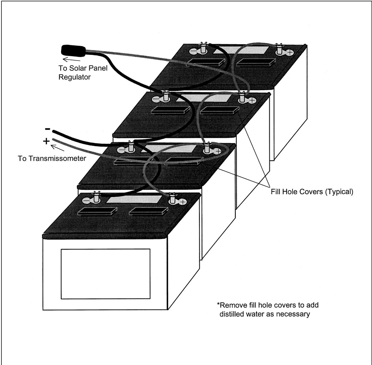
Figure 4-28. Deep-Cycle Battery and Interconnect Diagram.
