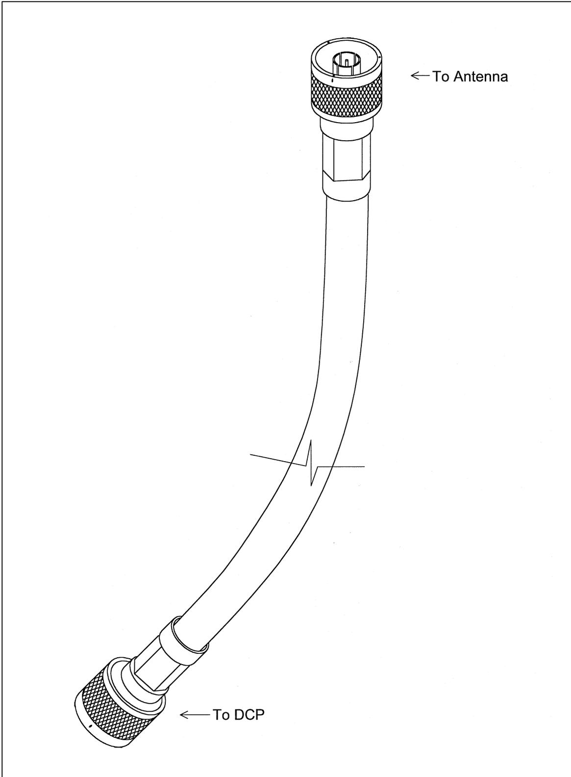
Figure 4-14. DCP Antenna Cable Connection Diagram.
