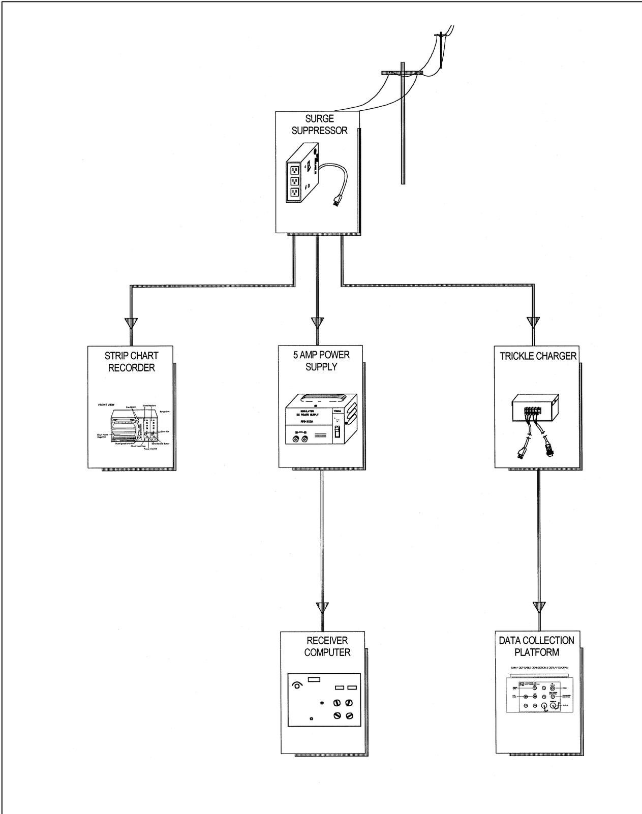
Figure 4-22. Receiver Station Line Power (AC) Configuration Diagram.
