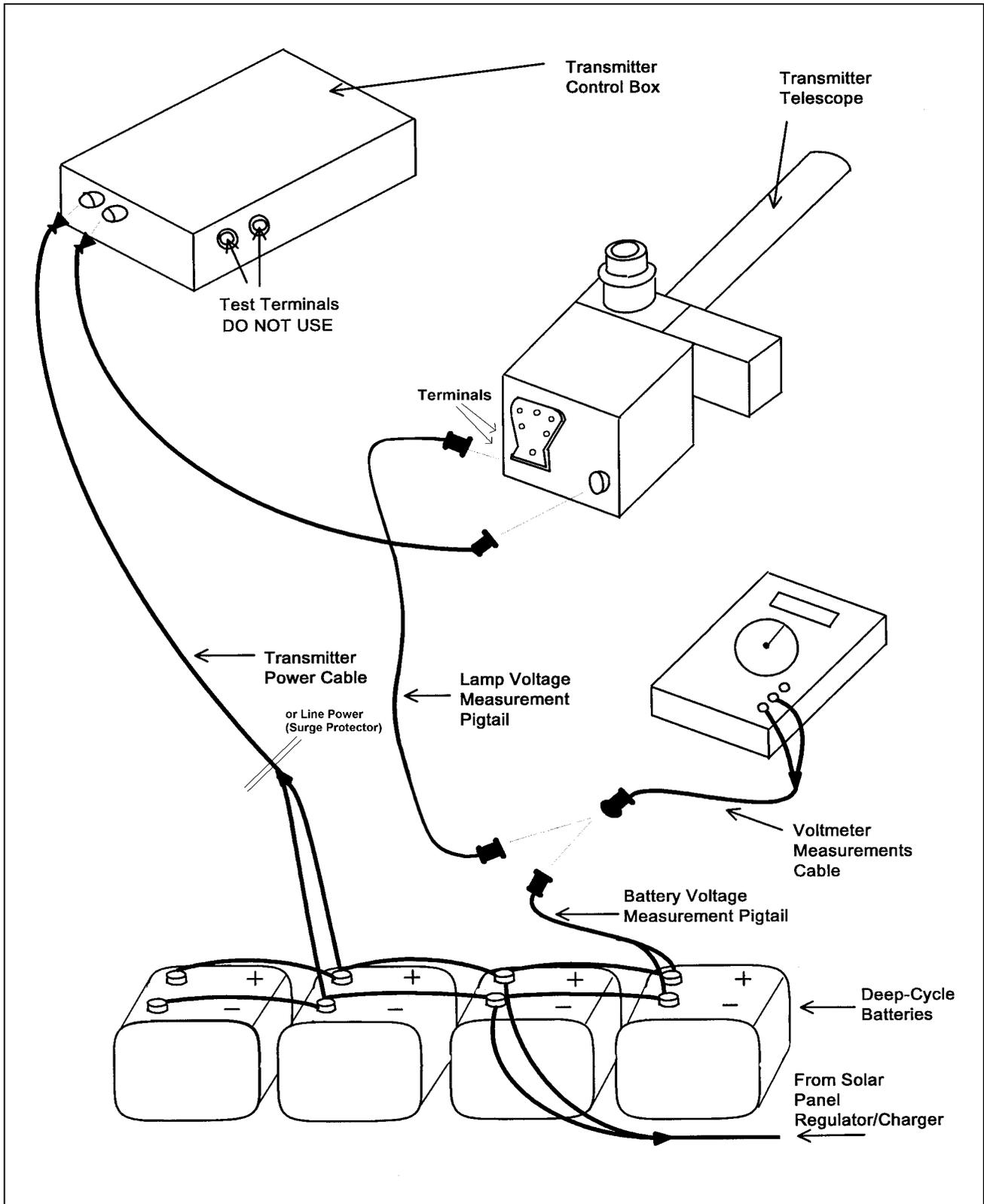
Figure 4-7. Transmitter Components Connection Diagram.
