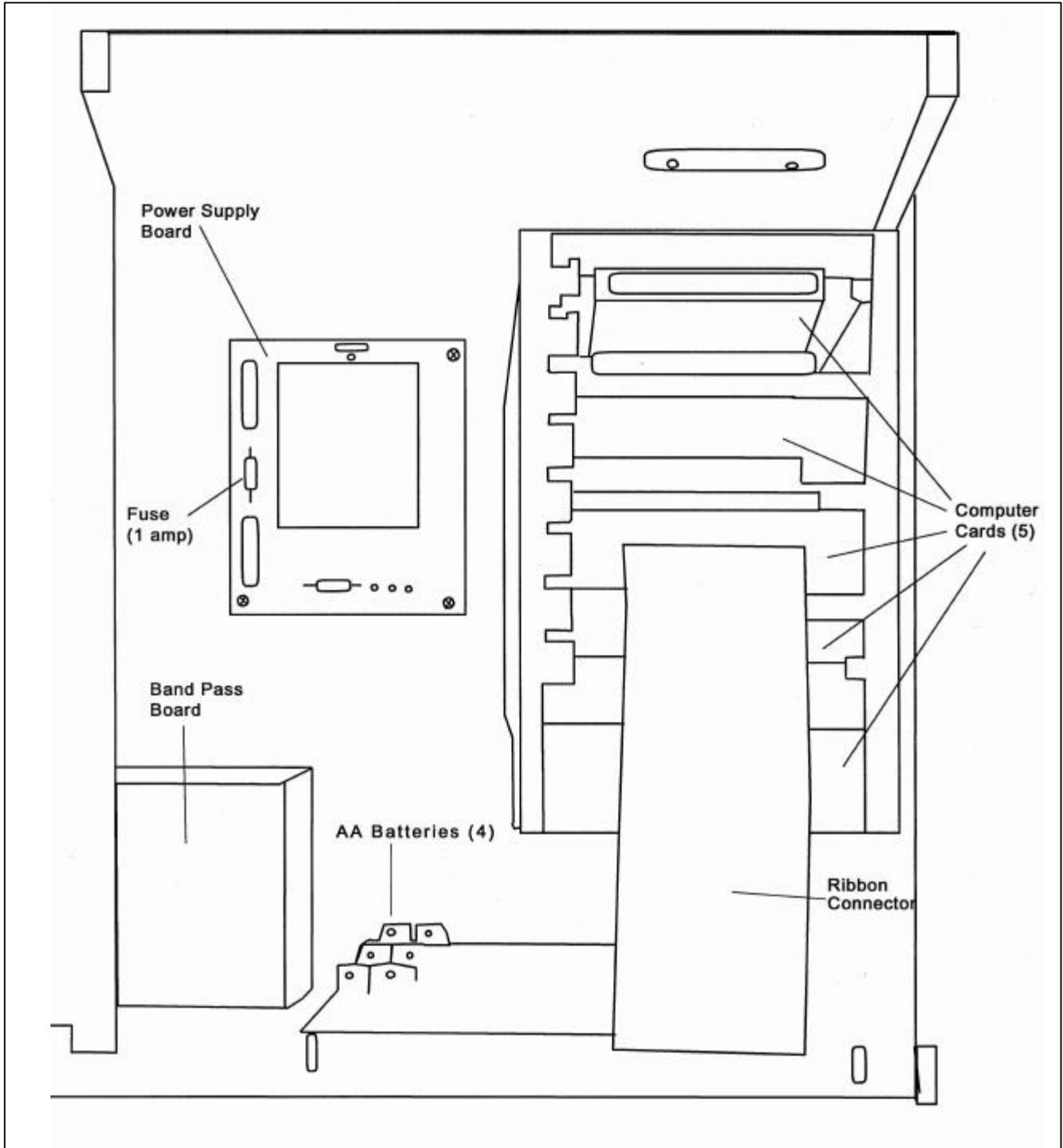
Figure 4-6. Receiver Computer Cards and Fuse Diagram.
