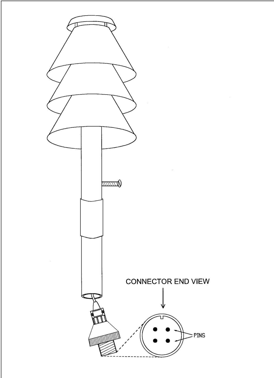
Figure 4-6. Air Temperature/Relative Humidity Sensor Component Diagram.
