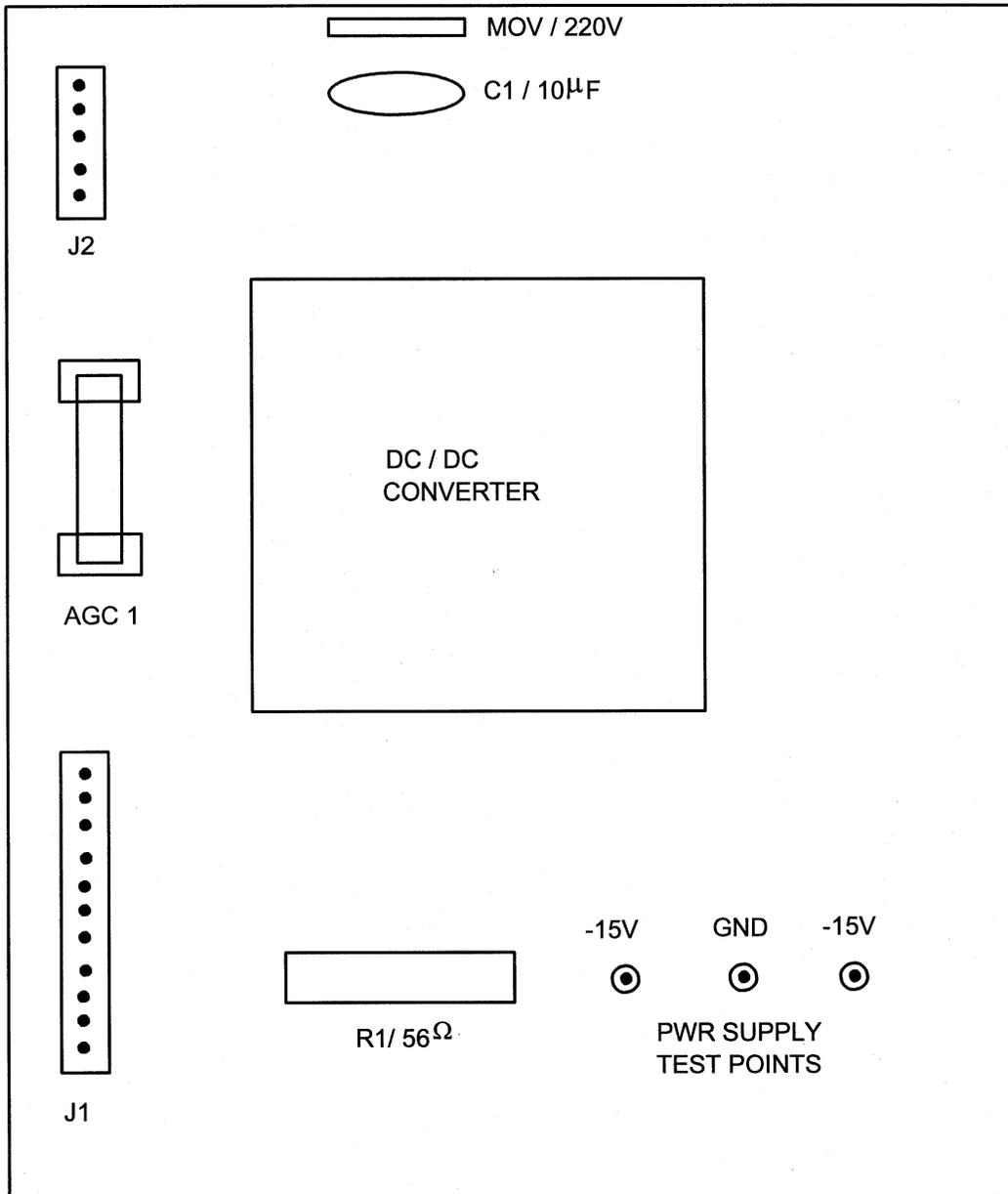
Figure 4-5. Power Supply Circuit Board Components Diagram.
