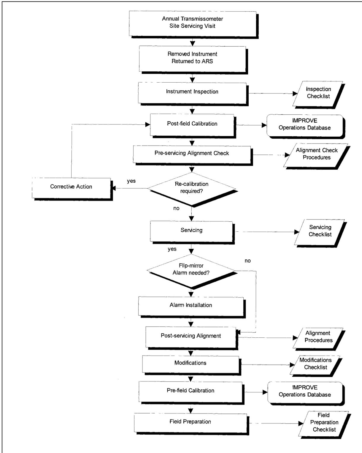
Figure 4-2. Annual Service Procedure for Optec LPV-2 Transmissometers.
