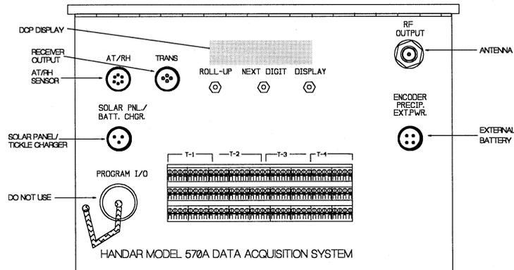
Figure 4-12. DCP Cable Connection and Display Diagram.
