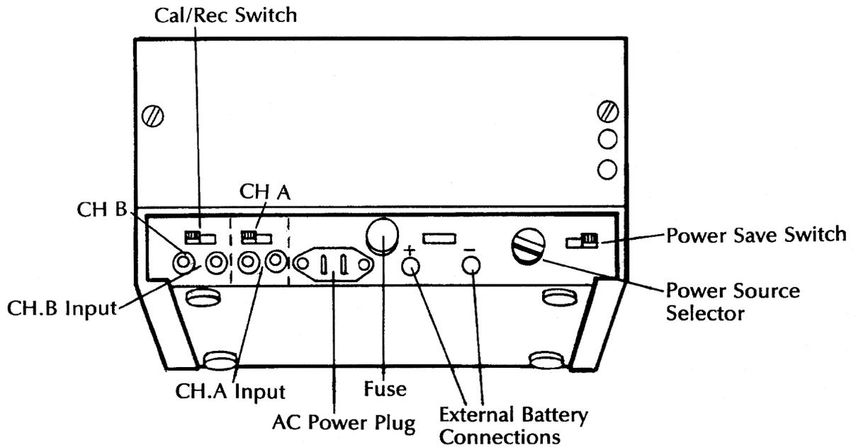
Figure 4-15. Strip Chart Component Diagram.
