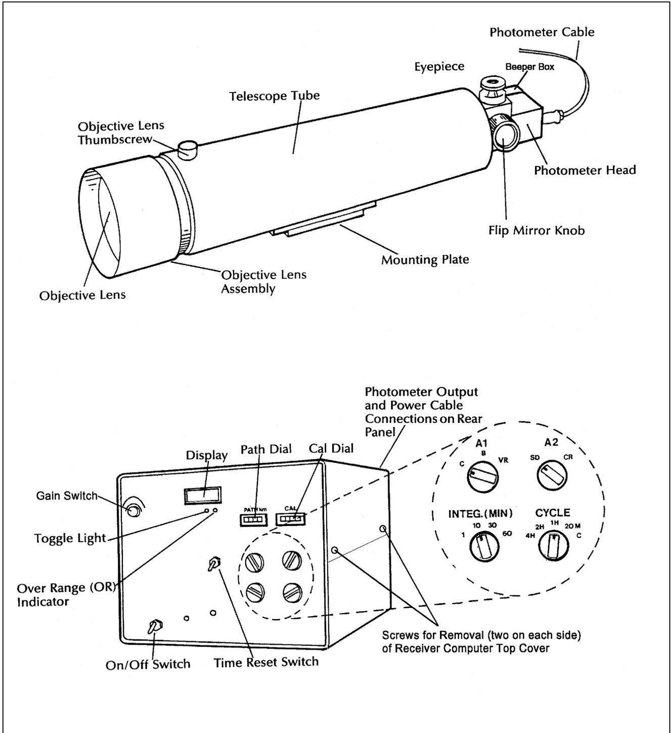
Figure 4-4. Receiver Component Diagram.
