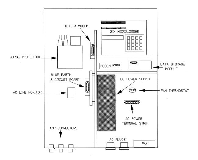
Figure 4-5. Datalogging and Support Subsystem Component Diagram.
