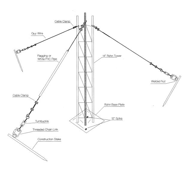
Figure 4-1. Nephelometer Tower Components.
