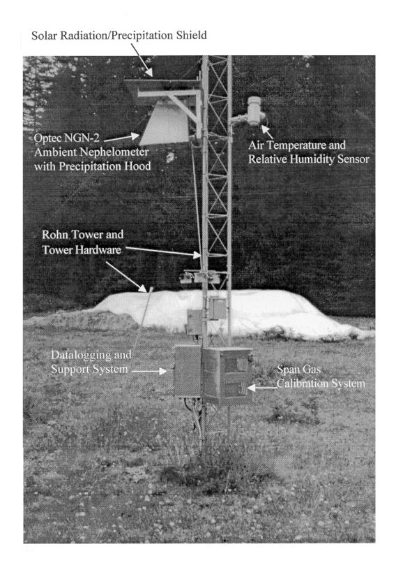
Figure 1-1. Typical Optec NGN-2 Nephelometer Station.
