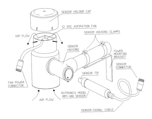
Figure 4-7. Rotronics AT/RH Sensor in Force-Aspirated Shield.
