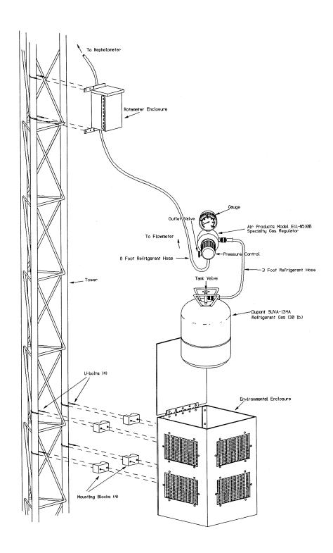
Figure 4-8. Span Gas Calibration System.
