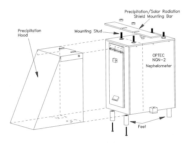
Figure 4-3. Precipitation Hood Installation Diagram.
