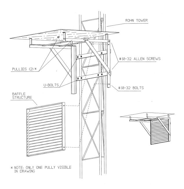
Figure 4-2. Solar Radiation and Precipitation Shield Assembly.
