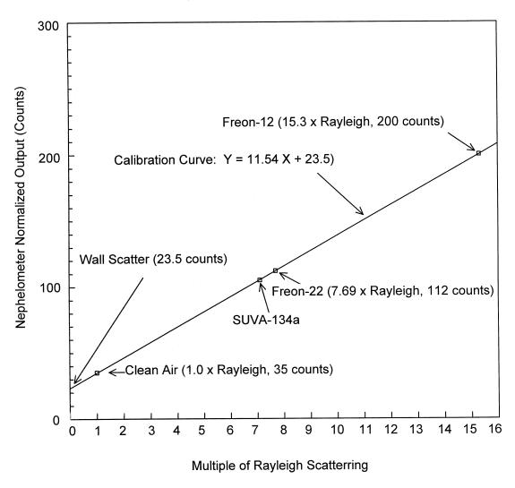
Figure A-1. Example Optec NGN-2 Calibration Curve.
