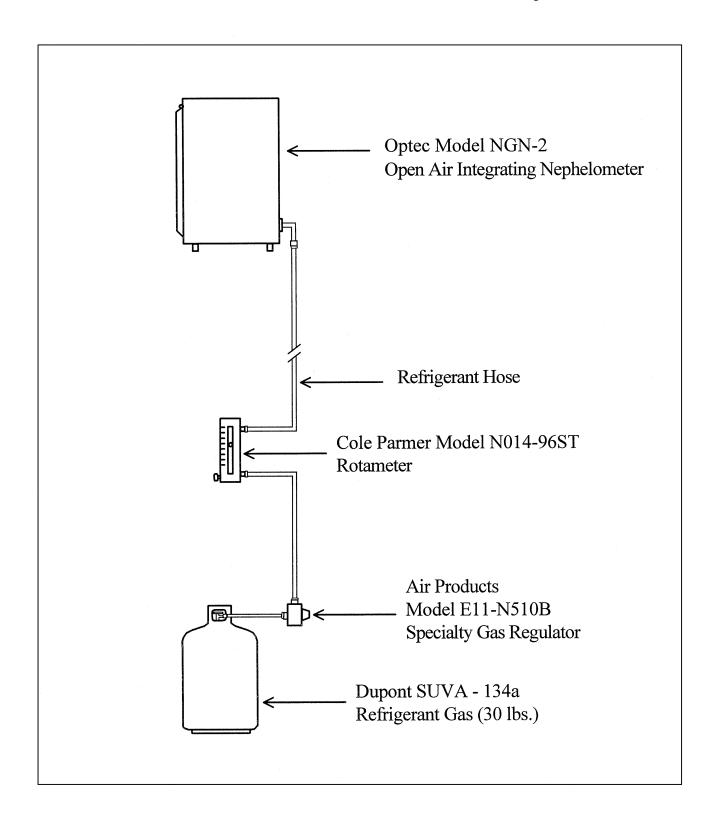
Figure 3-1. Manual Span Gas Calibration/Audit Configuration for the Optec NGN-2 Nephelometer.
