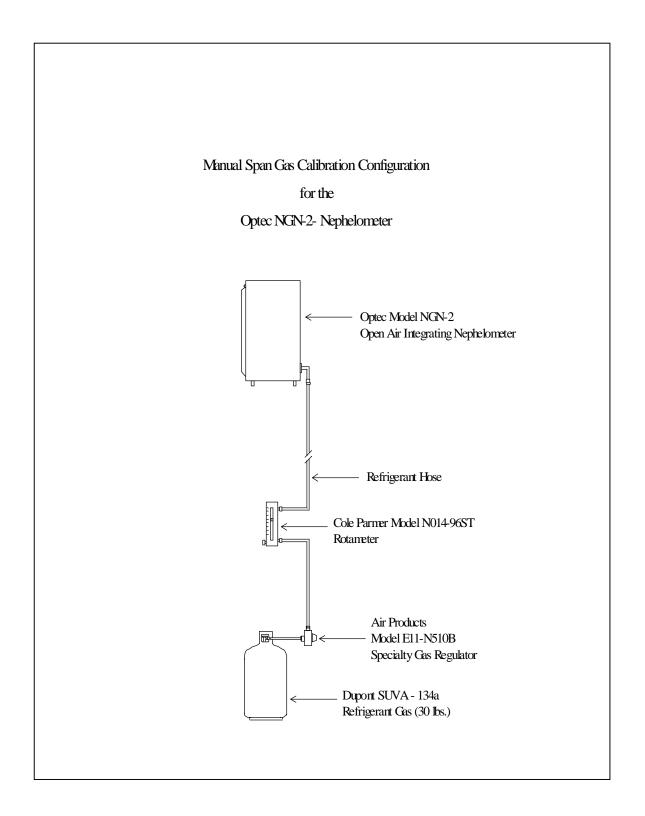
Figure 3-1. Manual Span Gas Calibration/Audit Configuration for the Optec NGN-2 Nephelometer.
