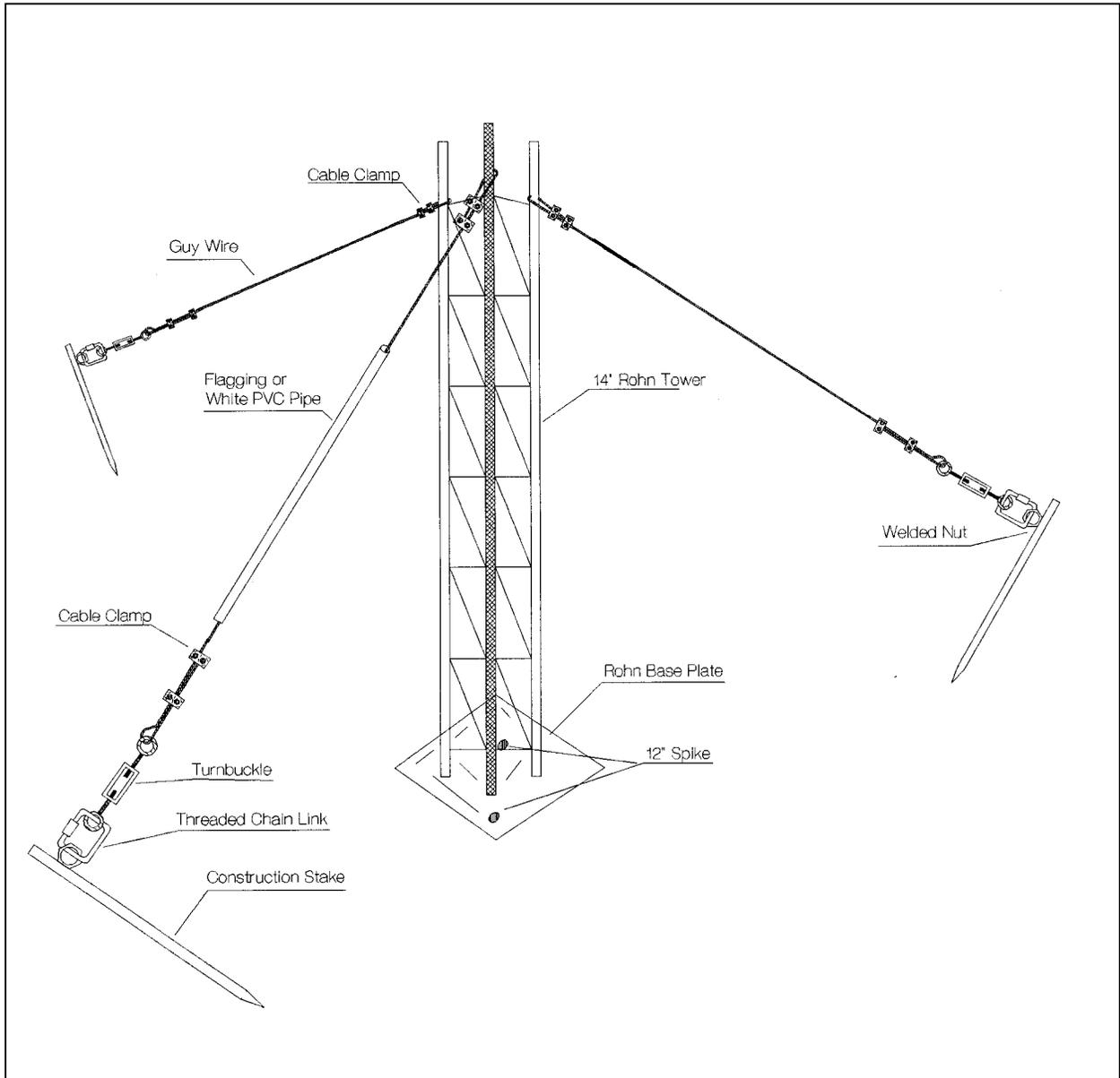
Figure 4-11. Nephelometer Support Tower and Related Hardware.
