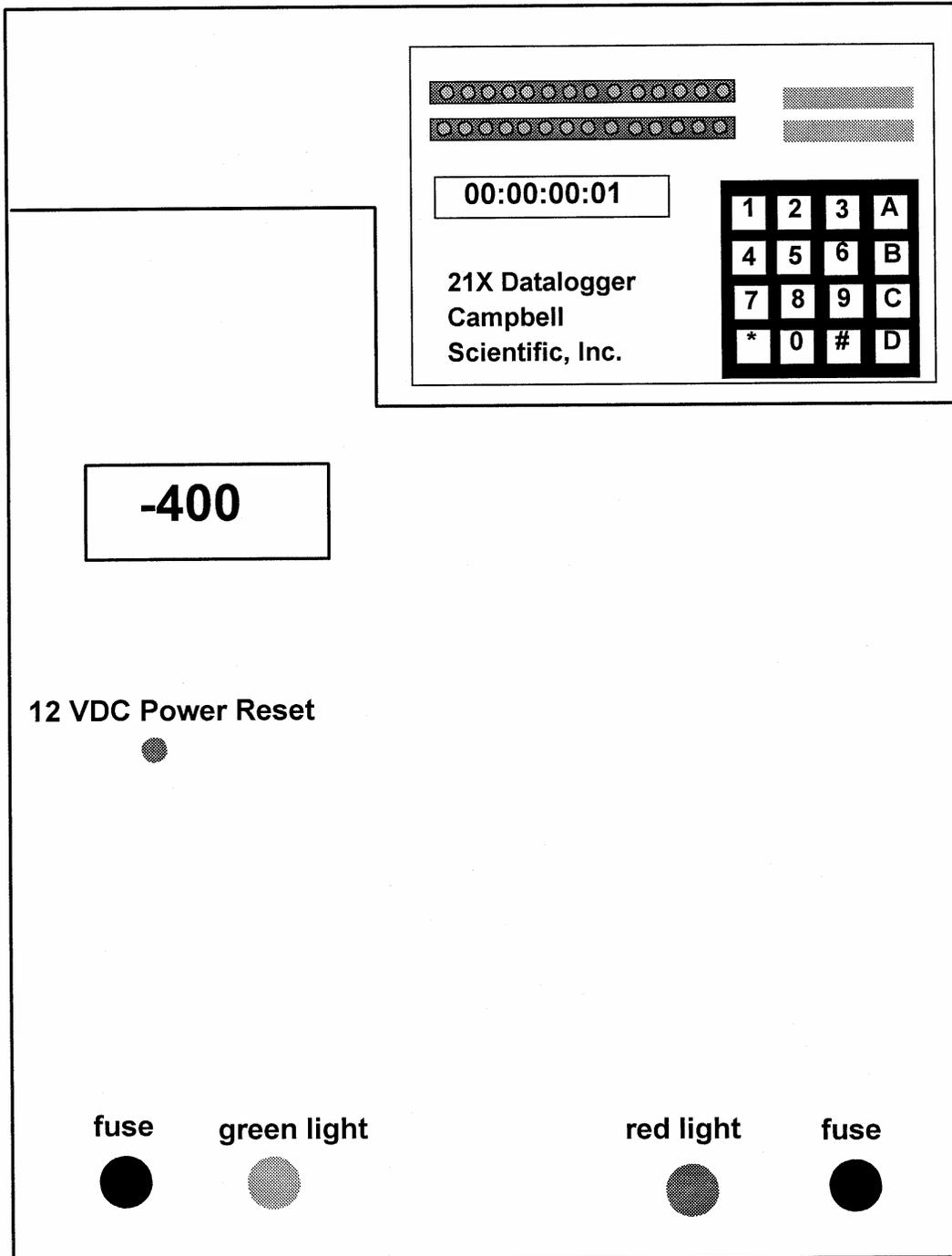
Figure 4-3. Datalogger Support System Front Panel.
