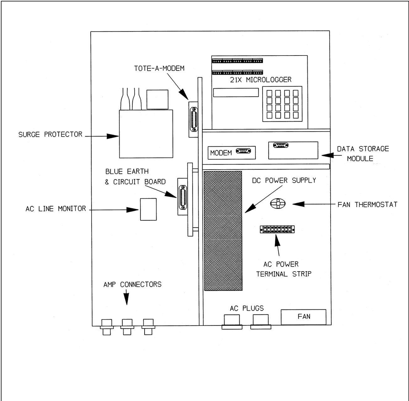
Figure 4-4. Data Logging and Control Subsystem Component Diagram.
