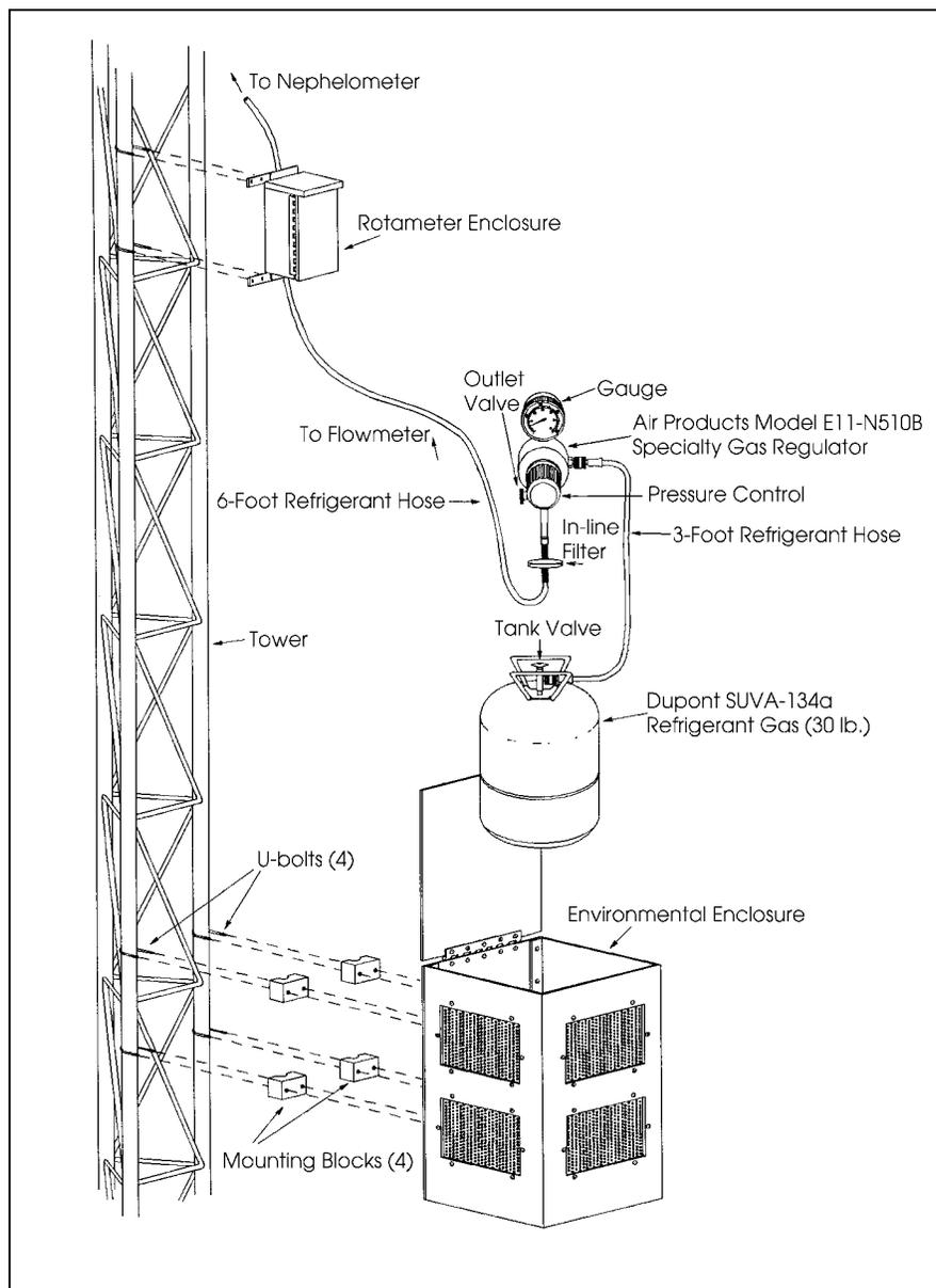
Figure 4-3. Span Gas Calibration System.
