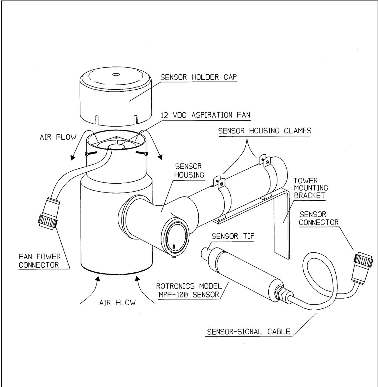
Figure 4-10. Rotronics AT/RH Sensor in Force-Aspirated Shield.
