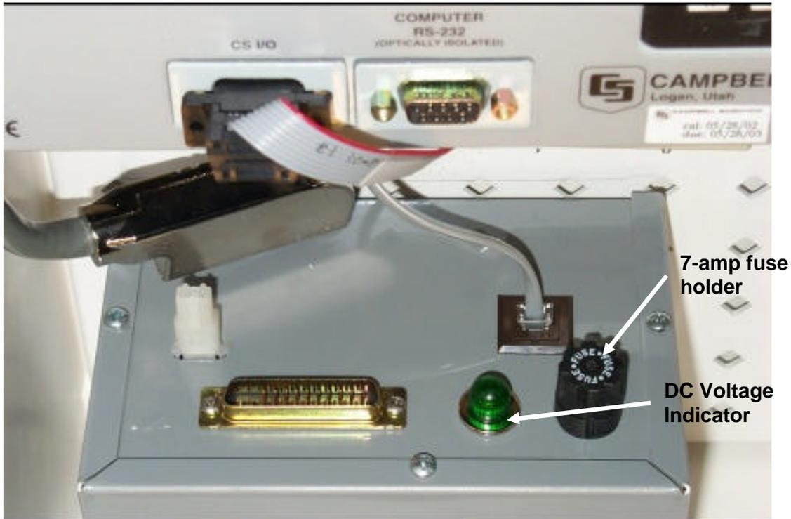
Figure 4-2. Junction Box Connector Panel in Support System.
