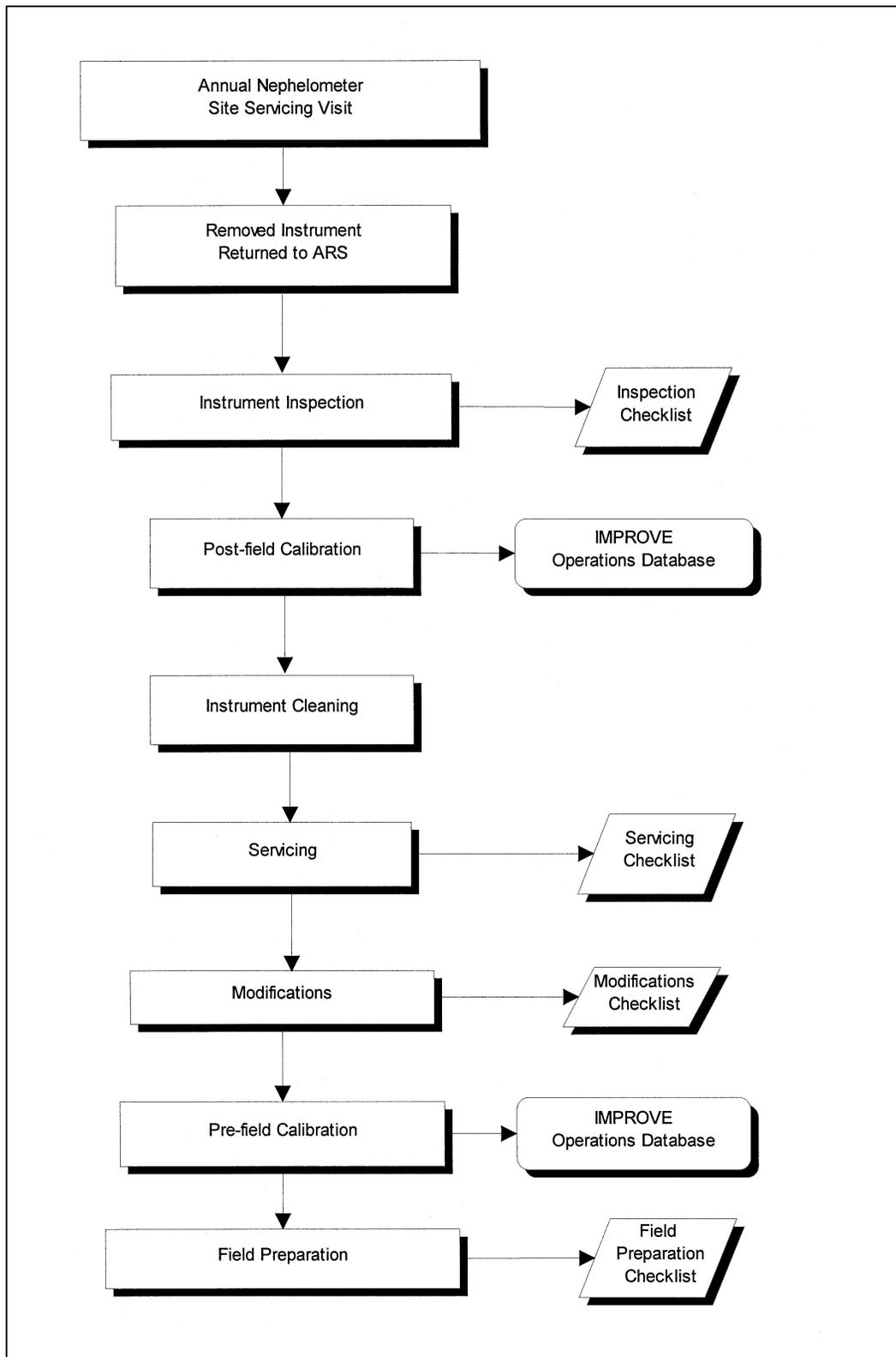
Figure 4-2. Annual Service Procedure for Optec NGN-2 Nephelometers.
