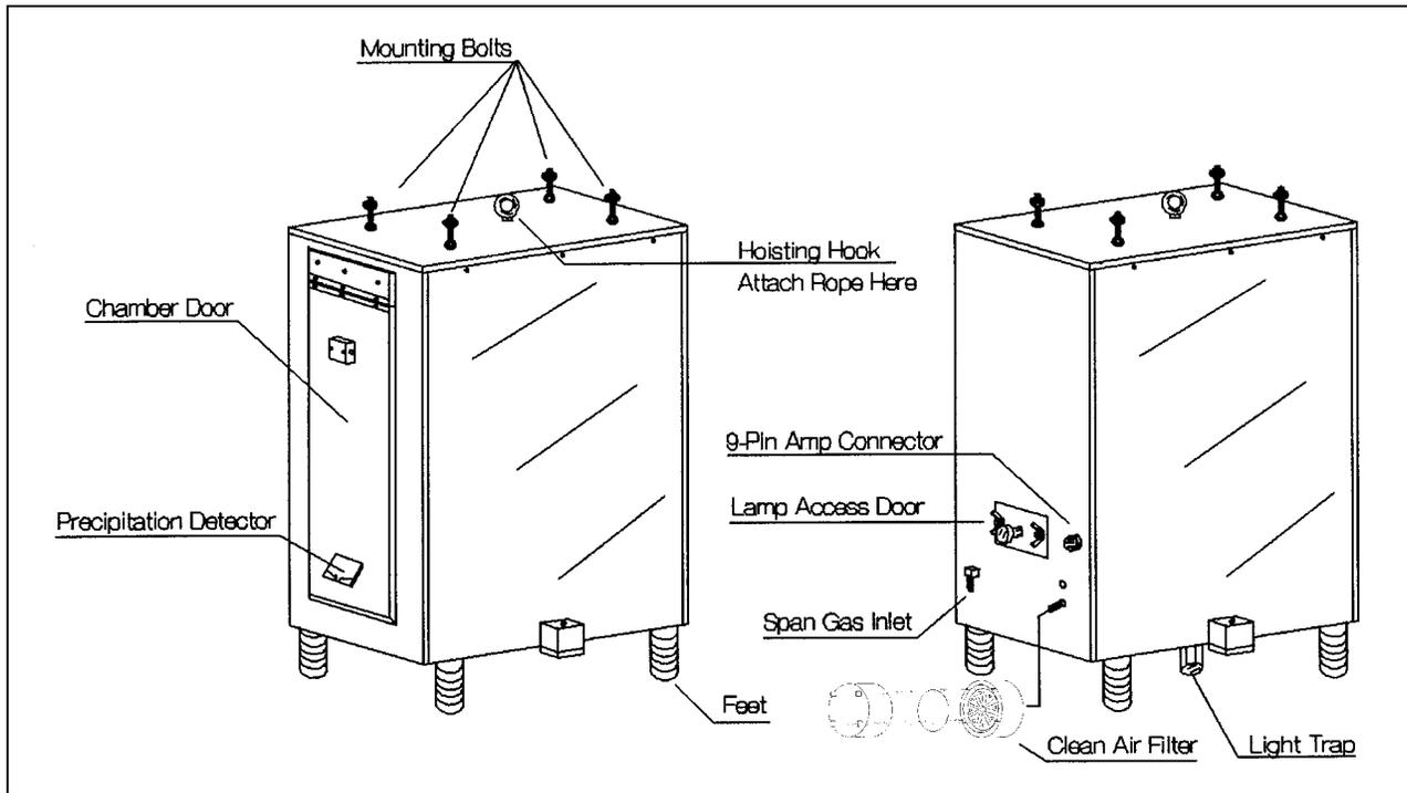
Figure 4-1. Optec NGN-2 Nephelometer Exterior Diagram.
