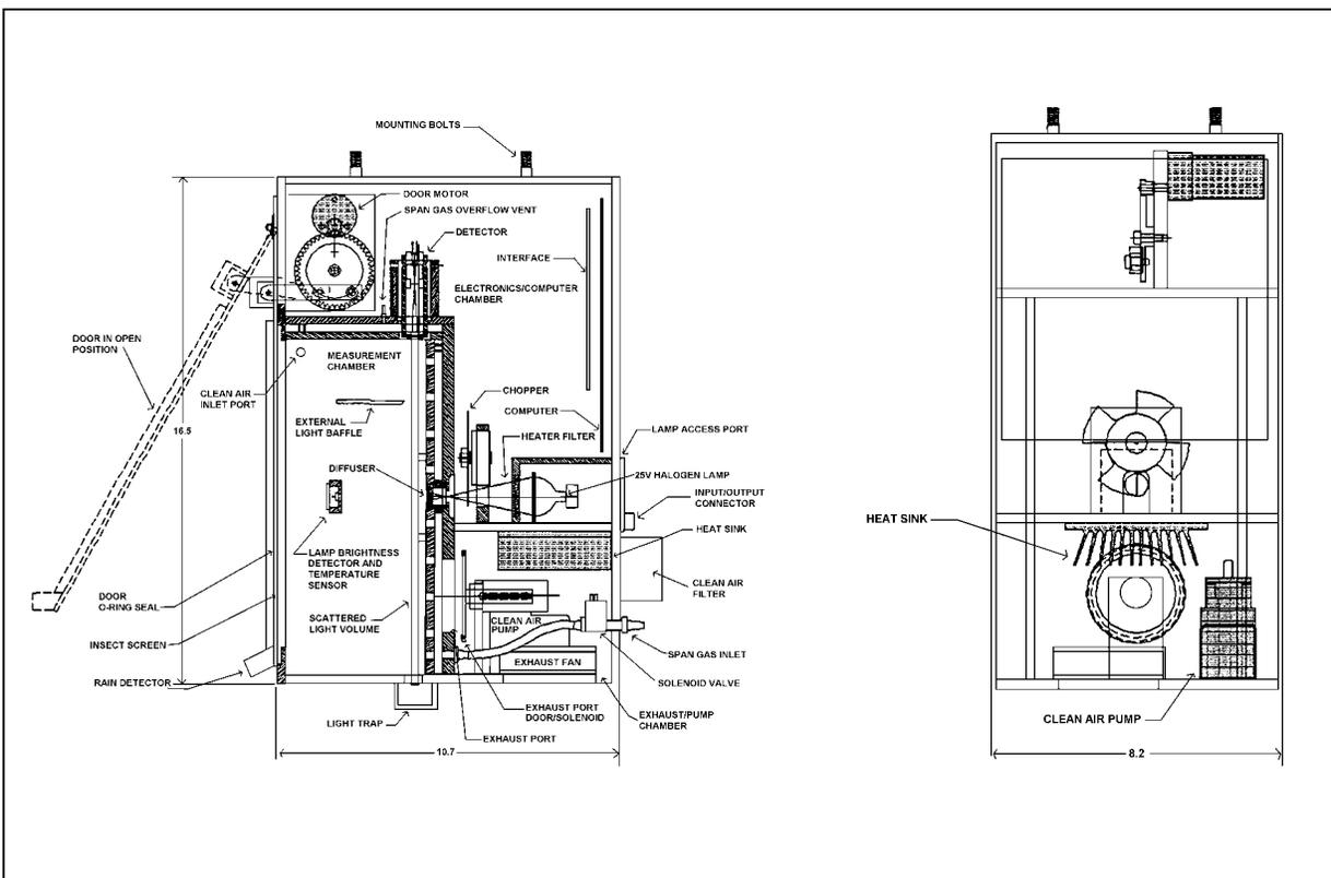
Figure 4-2. Optec NGN-2 Nephelometer Cross-Sectional View.
