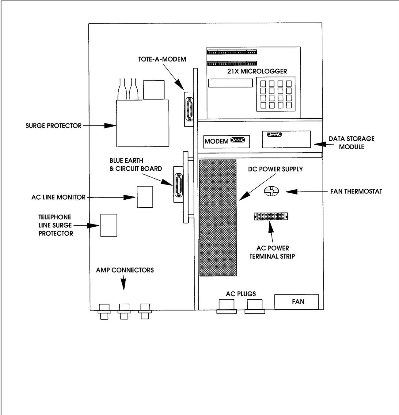
Figure 4-4. Data Logging and Control Subsystem Component Locations.
