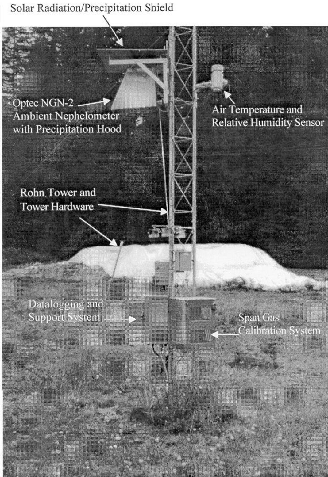
Figure 4-1. Typical Optec NGN-2 Nephelometer Station.
