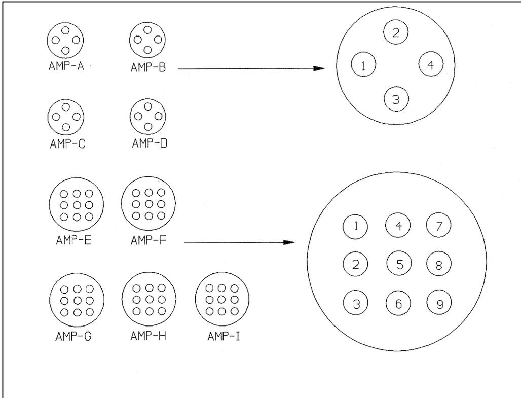
Figure 4-7. Data Logging and Control Subsystem Connector Panel Diagram
