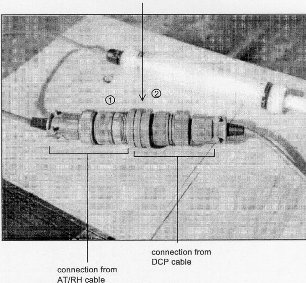
Figure 4-6. AT/RH Sensor/DCP Cable Connection Diagram.
