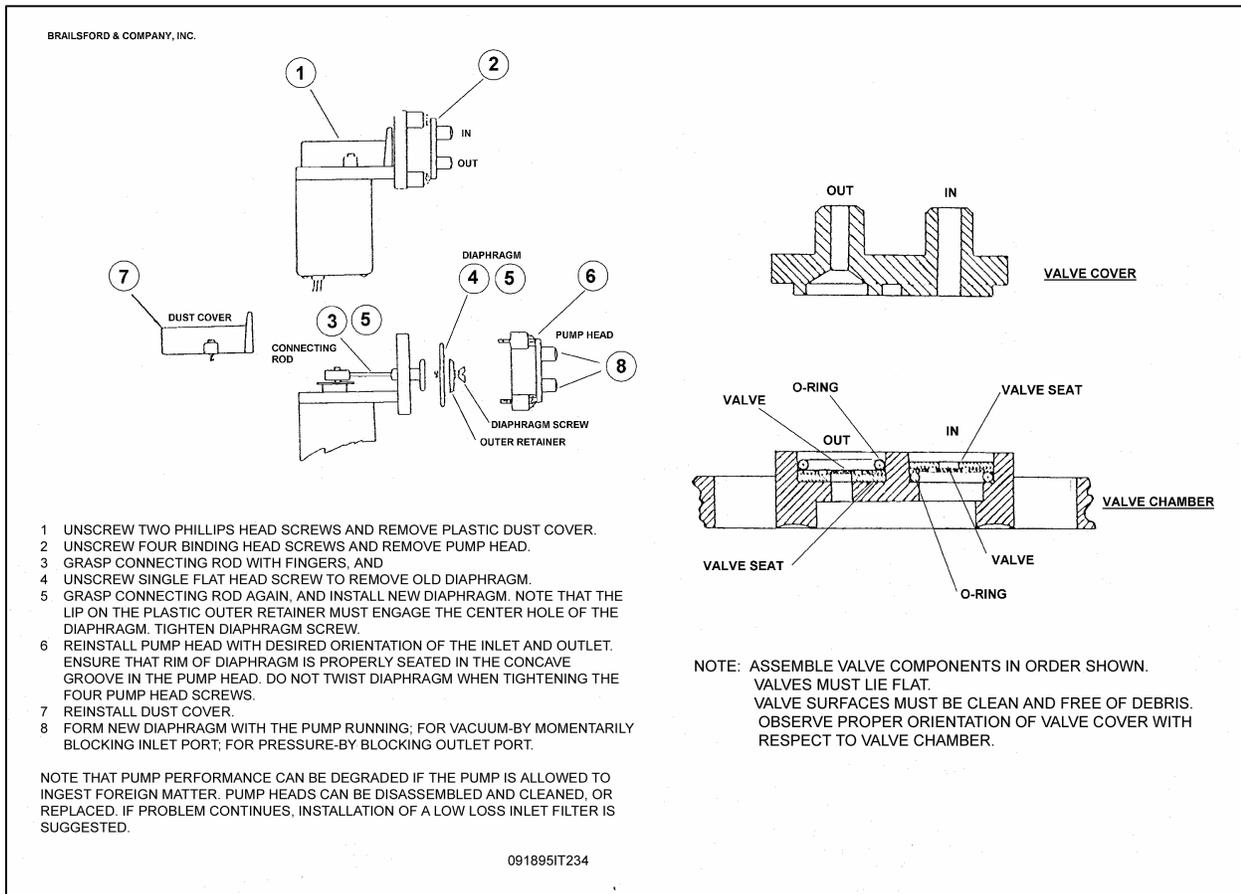
Figure 4-3. Brailsford Clean Air Pump Diaphragm and Valves.
