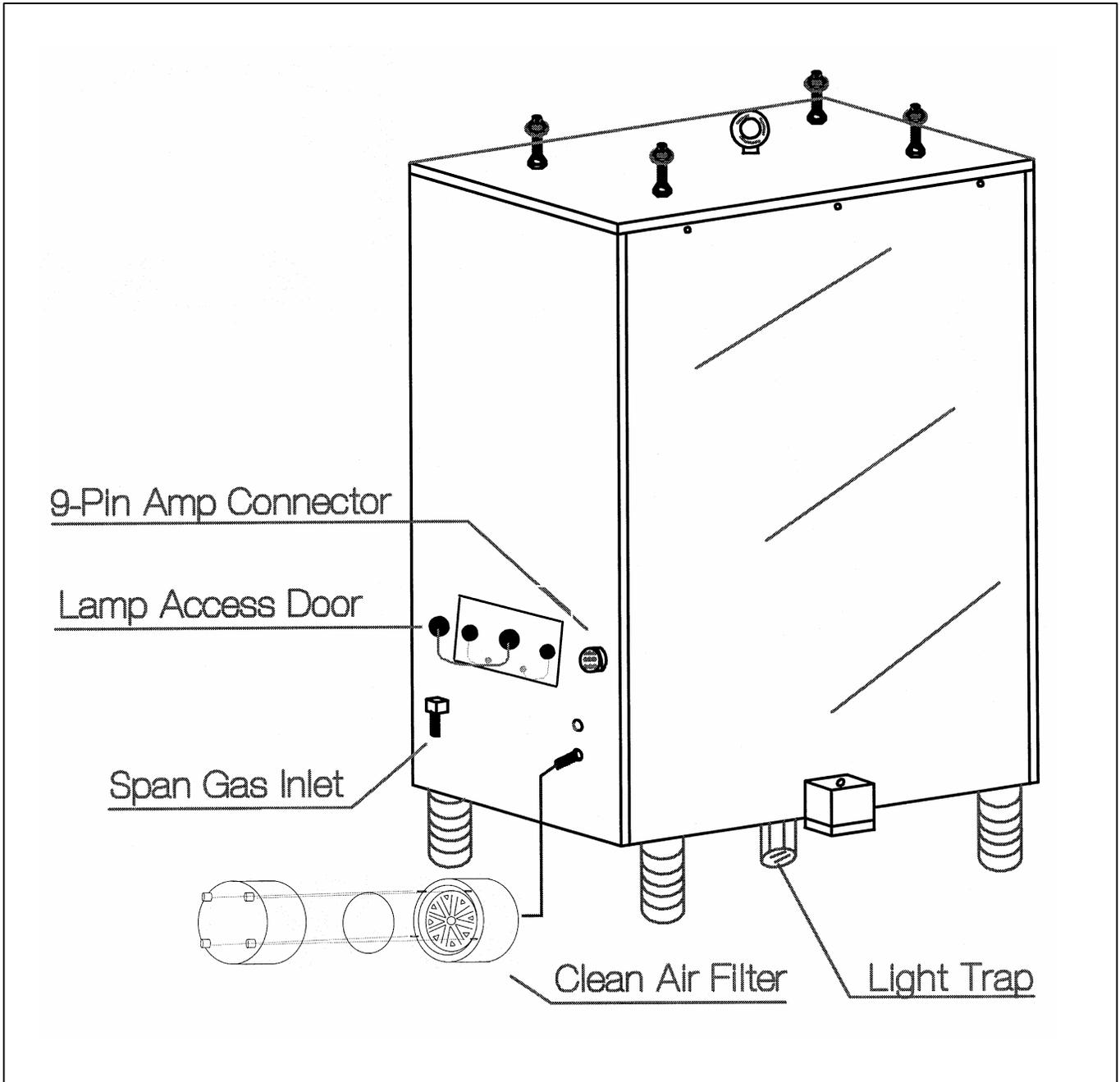
Figure 4-4. Diagram of the Clean Air Filter Assembly and Light Trap.
