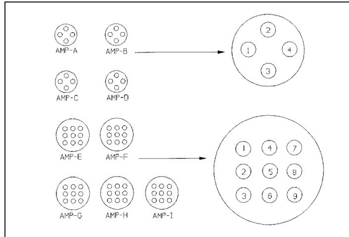
Figure 4-5. Data Logging and Control Subsystem Connector Panel.
