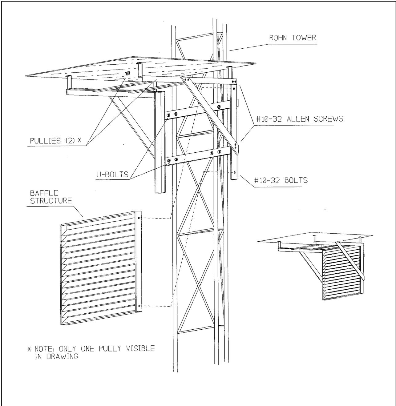
Figure 4-12. Precipitation and Solar Radiation Shield for Optec NGN-2 Nephelometer.
