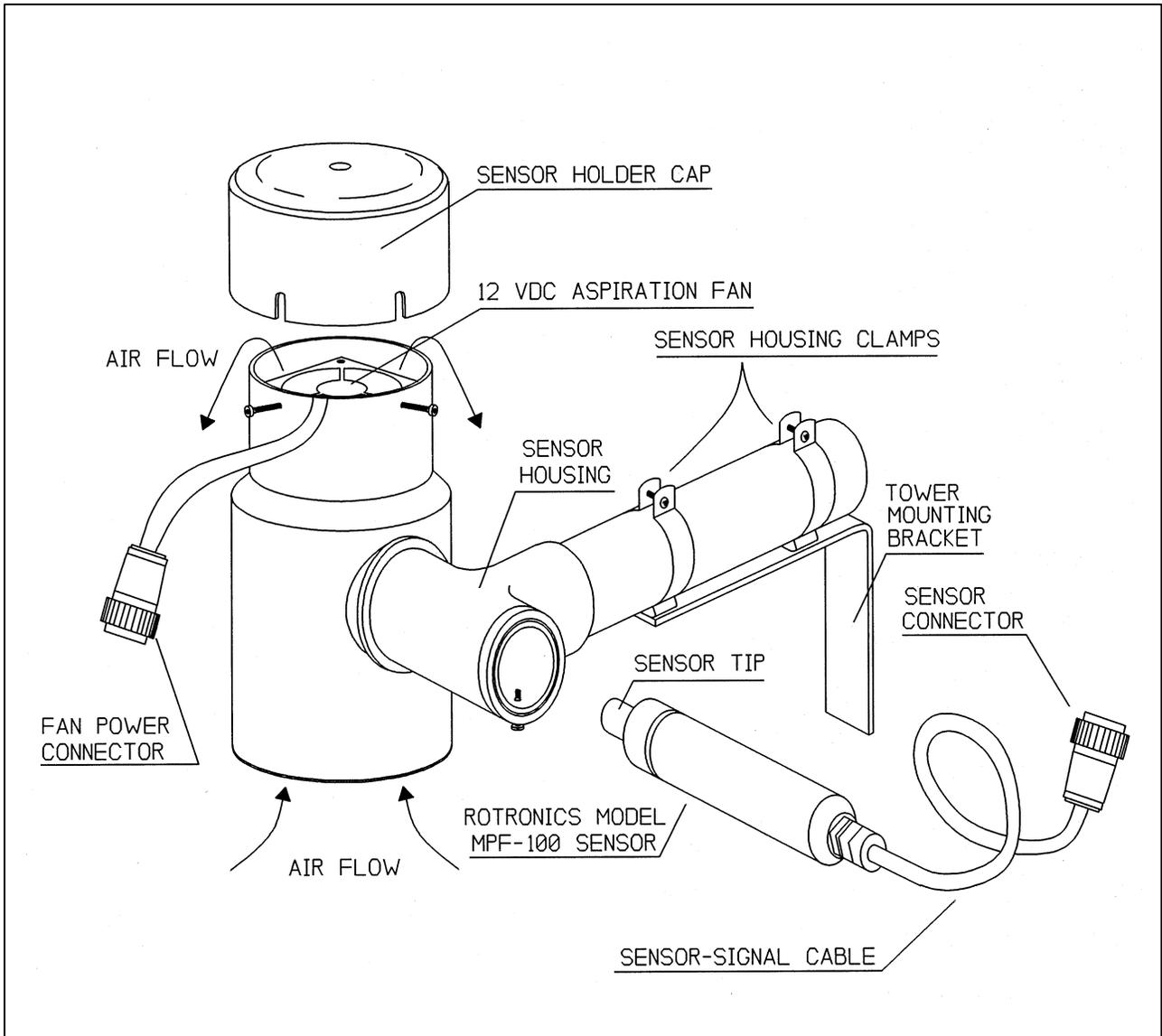
Figure 4-5. Rotronics Air Temperature/Relative Humidity Sensor Component Diagram.
