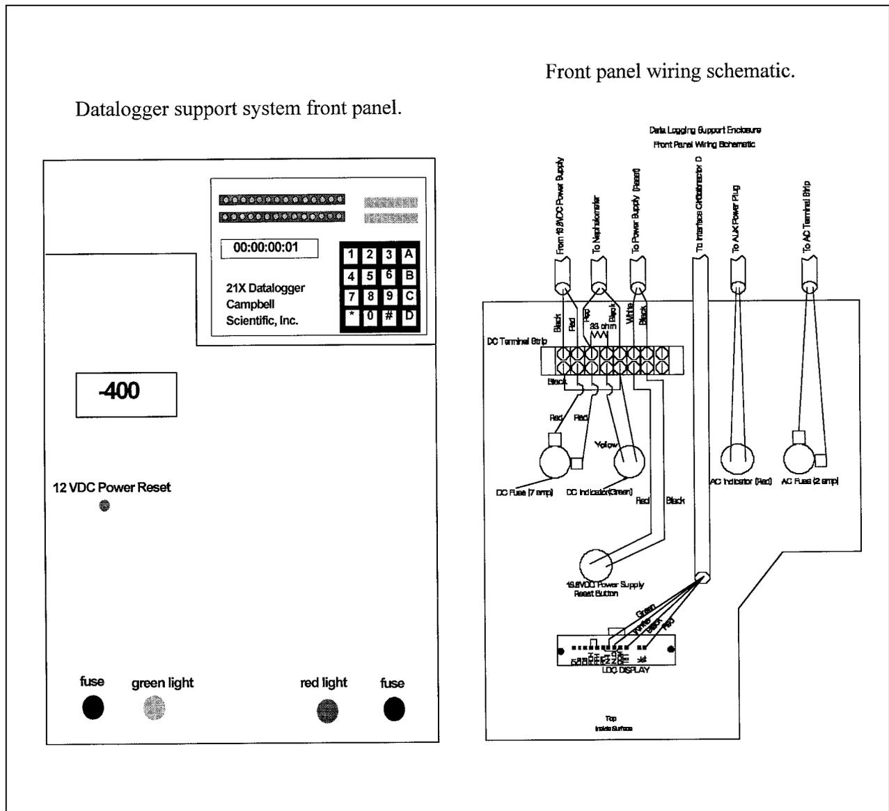
Figure 4-7. Datalogger Support System Front Panel.
