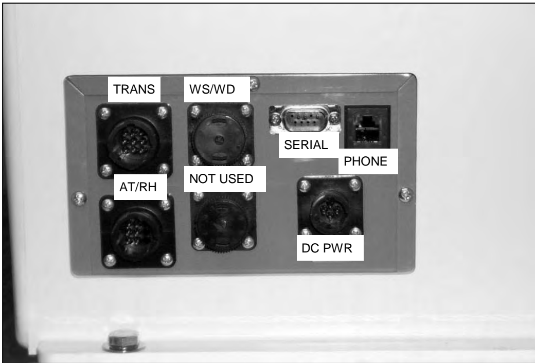
Figure 4-9. Datalogging and Control Subsystem Connector Panel.
