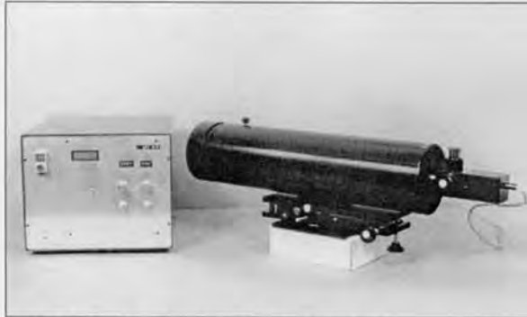
LPV-2 and LPV-3 receiver telescope and computer.
