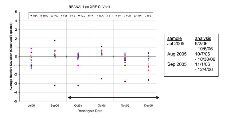
**Figure 7.** Reanalyses of REANAL1 samples on XRF-Cu system. Horizontal arrow indicates when Jul-Sep 2005 network samples were analyzed.
