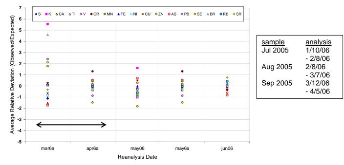
**Figure 6.** Reanalyses of REANAL2 samples on XRF-Mo system. Horizontal arrow indicates when Jul-Sep 2005 network samples were analyzed.
