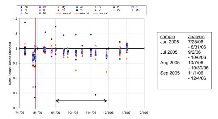
Figure 2. XRF-Cu system performance chart based on standards.
