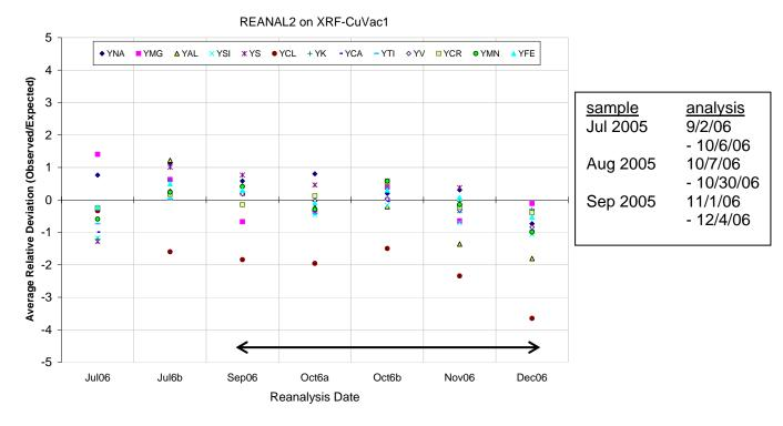
**Figure 8.** Reanalyses of REANAL2 samples on XRF-Cu system. Horizontal arrow indicates when Jul-Sep 2005 network samples were analyzed.
