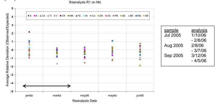
**Figure 5.** Reanalyses of REANAL1 samples on XRF-Mo system. Horizontal arrow indicates when Jul-Sep 2005 network samples were analyzed.
