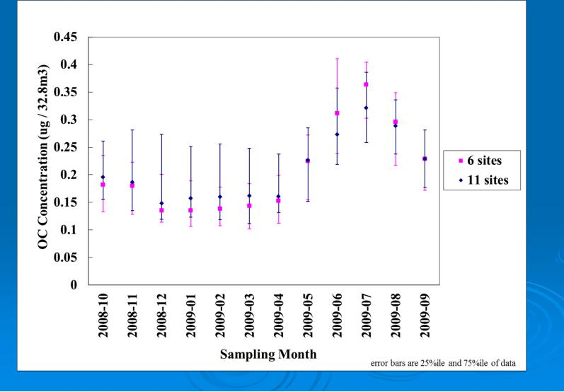
Estimating Quantitative Limit for OC with Monthly Median Artifact Correction One year of data > 11 sites with back filters For each sample calculate • Sample specific OC, best estimate  $OC_{ss} = (front - back)/air volume$  Monthly median corrected OC  $OC_{mm} = (front - back_{mm})/(air volume)$ Back<sub>mm</sub> = median from 10 other sites This is the method used for most sites in **IMPROVE** for the carbon fractions
