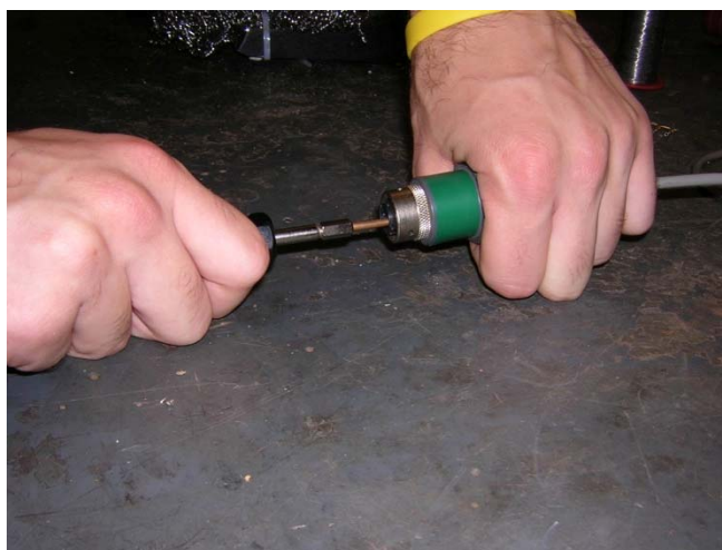
Figure 28. Removing the Connector Pins.
