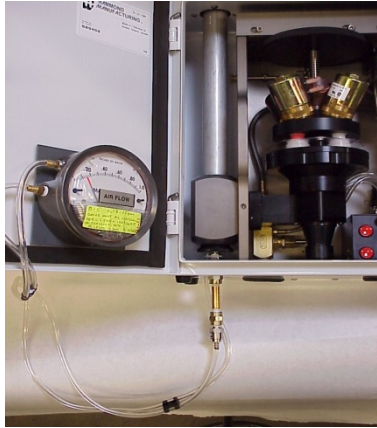
Figure 2. Inserting the Probe into the Tee
