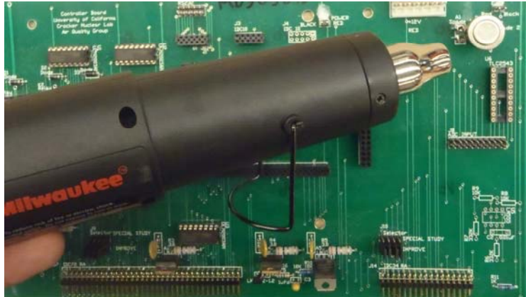
Figure 10. Thermostat Being Heated with Heat Gun
