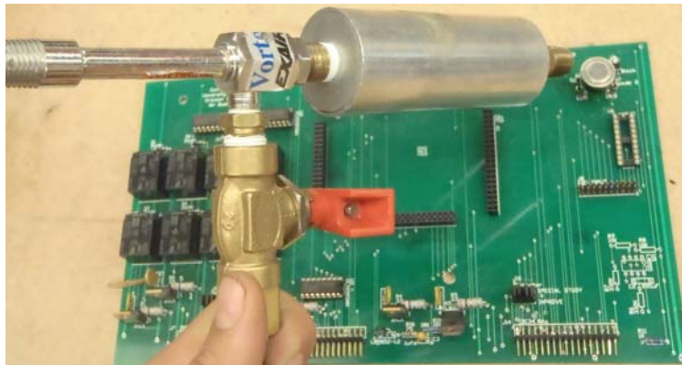
Figure 11. Thermostat Being Cooled with a Vortex Tube
