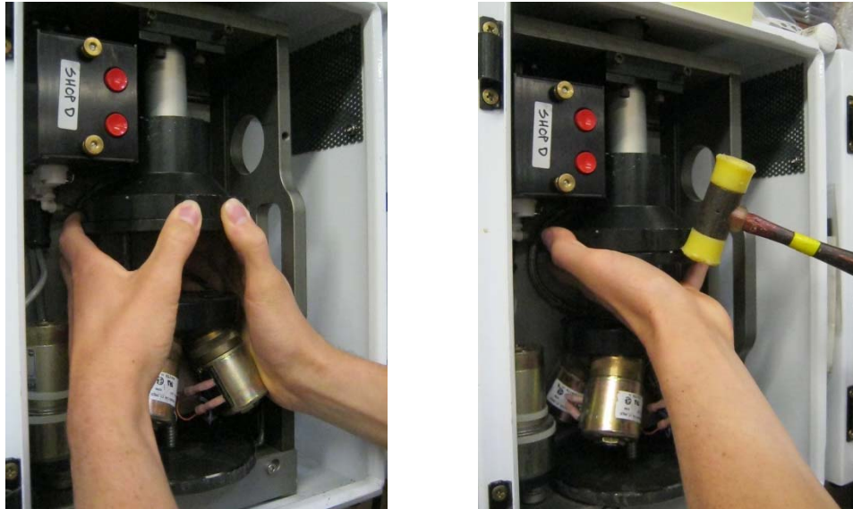
Figure 7. Removing the Bottom Lid of Module "D"
