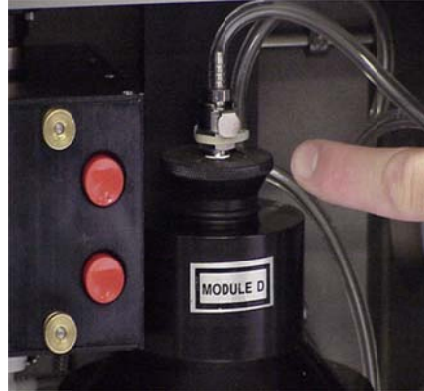
Figure 6. Placing the Probe in Module "D" (con.)
