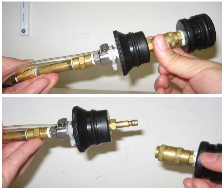
Figure 4. Releasing the Probe Plug
