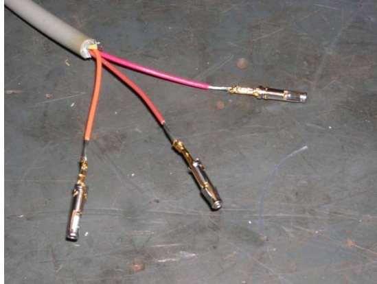
Figure 25. Wires with Pin Attached.
