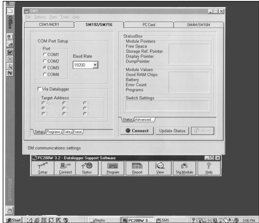
Figure 4-2. SMS Screen Setup (Com Port and Baud Rate).
