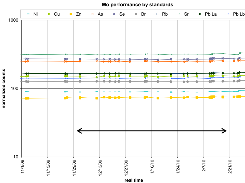
Figure 1B. Mo XRF system performance chart based on normalized counts.
